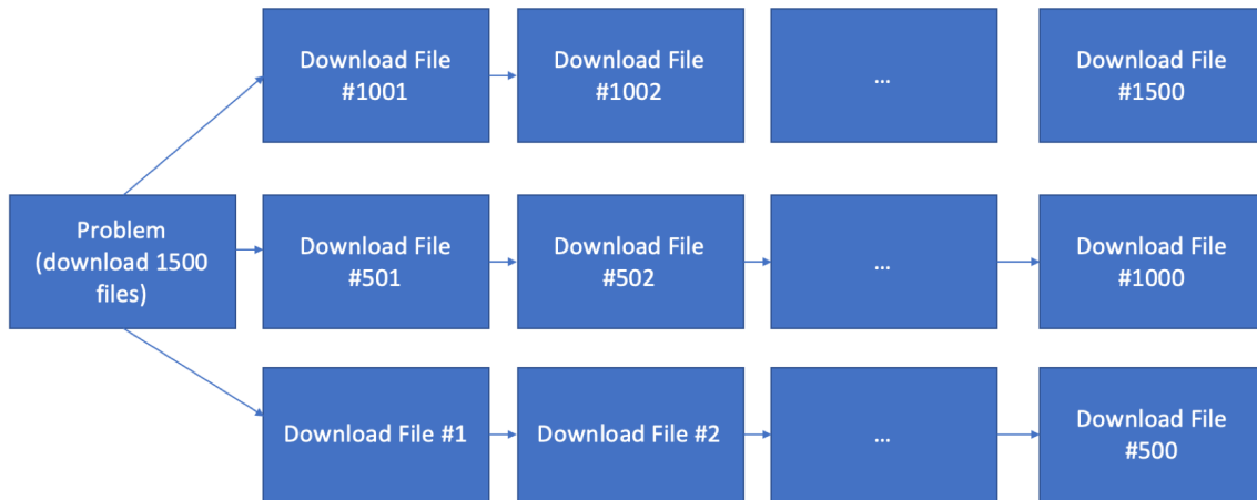
Figure 6.2 This view shows an example of a parallelization workflow for downloading the same example 1500 files. Here, we can split up the downloads into separate workflows that occur at the same time. The benefit is that the original task of getting all of the files downloaded occurs much faster because multiple file downloads occur simultaneously in parallel.
