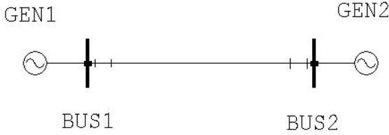
Fig. 8.5 Two-machines power system
