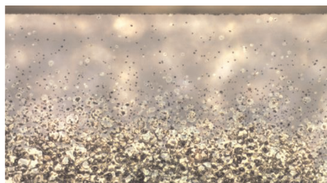
Figure 4. View of a fragment of the applied polymer layer (RR)-P 3 HT on the quartz crystal of the AFP module. View of the boundary of the formation of a porous layer from the crystal edge visible from above 100x magnification [1].
