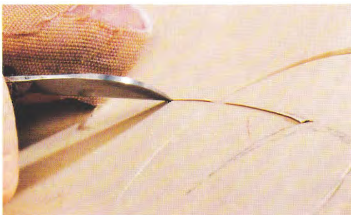
From there cut to the end of the stem lifting blade out of the wood to go over the previously cut leaf and continuing on the other side to the end.
