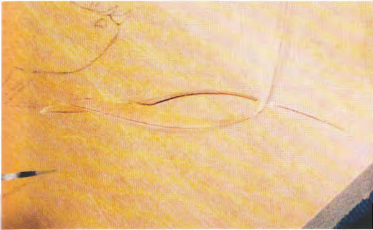
This meets the return line in a little more graceful way than a stop.
