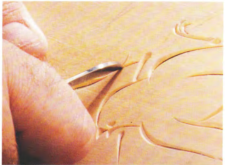
Turn the board and make the return cut.
