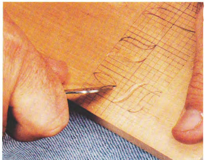
Start at the corner with the knife vertical and shallow.
