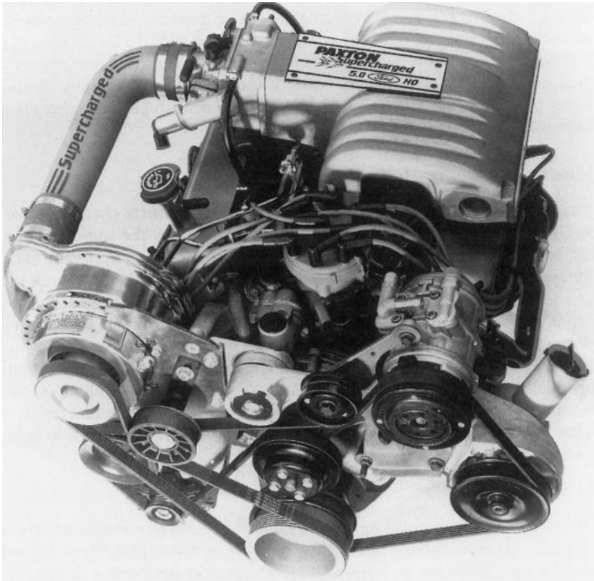
Figure 12a Installation of a centrifugal supercharger requires some revision of the belt drive system so it can be driven off the crankshaft pulley. (Courtesy Paxton Superchargers.)
