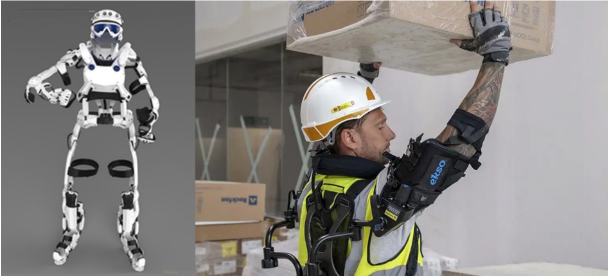
Figure 15.4 – Exoskeleton and robotic vest (sources: Clker and Scottish Construction Now)
