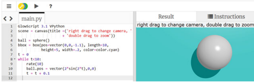
Fig. 1.5 Trinket (GlowScript) programming environment. Left: program editor; right: output window. The output is post-processed with POV-Ray to include ray tracing effects
