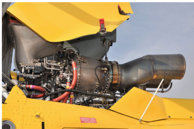
Fig. 34.4 Helicopter exhaust gas nozzle made of molybdenum steel (Photo Joaquim Sanz. MGVM)
