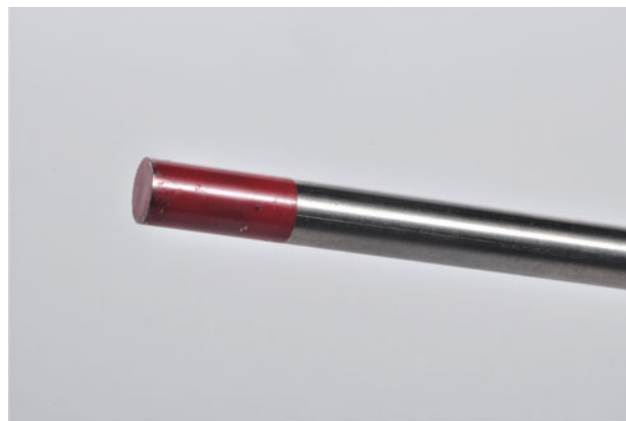
Fig. 57.3 Tungsten-thorium welding electrode. (Photo Joaquim Sanz, MGVM)
