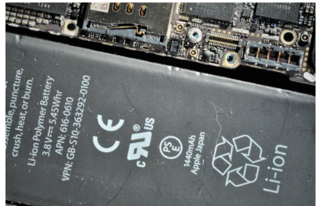
Fig. 30.4 Li-ion battery (Photo Joaquim Sanz. MGVM)
