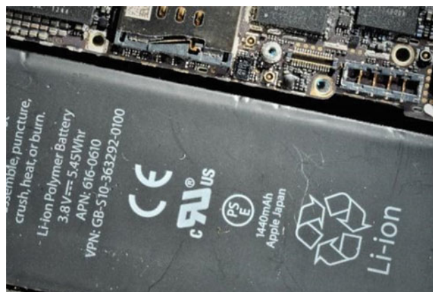
Fig. 18.4 Li-ion battery. (Photo Joaquim Sanz. MGVM)
