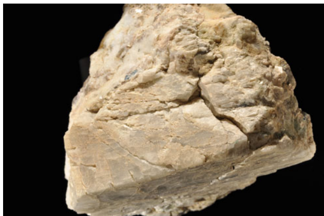
Fig. 30.1 Spodumene (aluminum and lithium silicate). Namibe (Moçâmedes) (Angola) (Photo Joaquim Sanz. MGVM)
