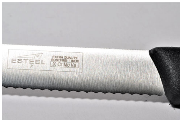
Fig. 34.3 Knife blade of alloy steel with molybdenum, chrome, and vanadium (Photo Joaquim Sanz. MGVM)
