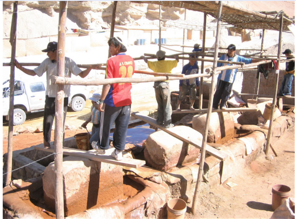
Fig. 3 Grinding rock by 'human force...' for the extraction of gold. Misky Mines (Camaná) (Perú) (Image courtesy of Silvia Palacios)
