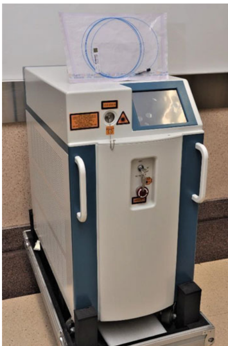
Fig. 71.3 Holmium laser equipment. (Photo Joaquim Sanz. MGVM)
