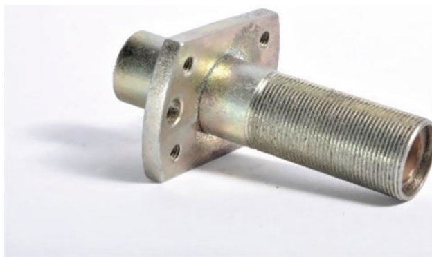
Fig. 10.4 Cadmium-plated steel. (Photo Joaquim Sanz. MGVM)
