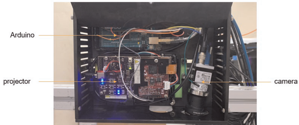
Figure 30. Actual internal image of the probe.
