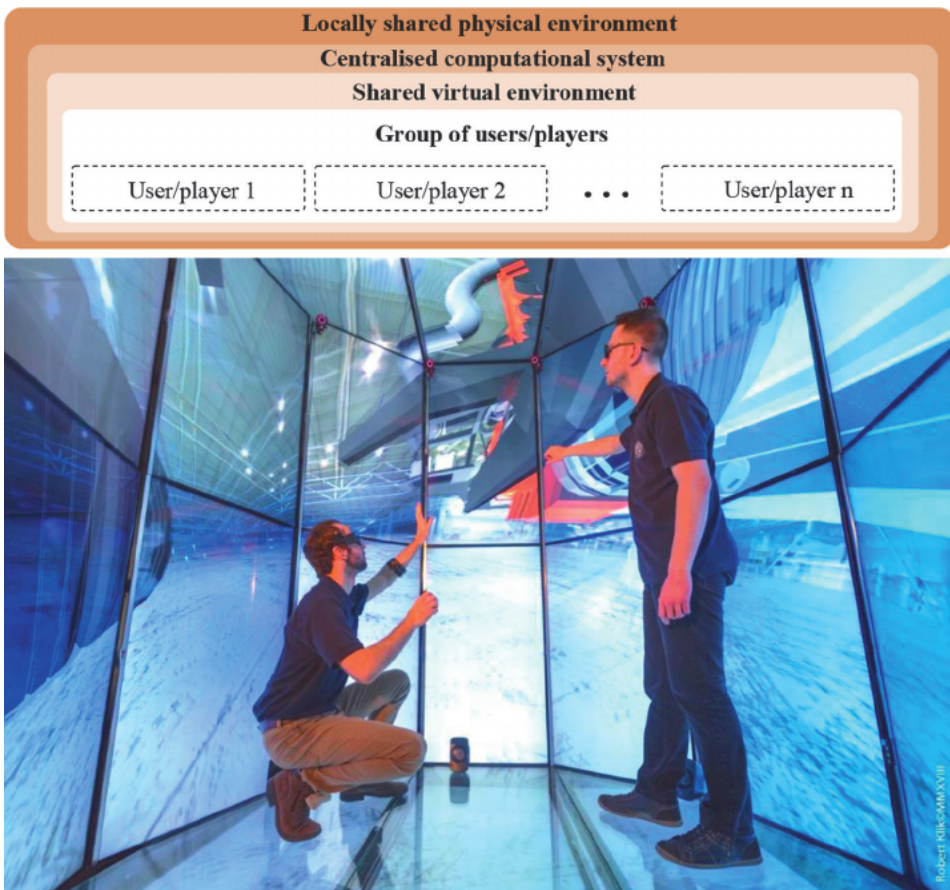
Figure 2. Locally shared environment with centralized user access (LIRKIS CAVE virtual cave environment).
