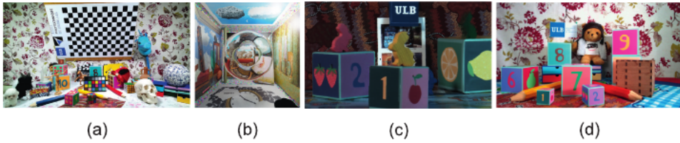
Figure 10. Overview of the open-source datasets. (a) Toystable consists of two camera arrays at 25 cm ( 5 \times 5 cameras) and 55 cm ( 3 \times 5 cameras) from the scene. (b) Magritte is a 21 \times 21 camera array. (c) Rabbit is a 3 \times 7 array of 5 \times 5 subaperture images of a plenoptic camera. (d) Bear ( 4 \times 8 cameras) is a dataset captured by a Lidar camera with estimated and sensed depth maps.
