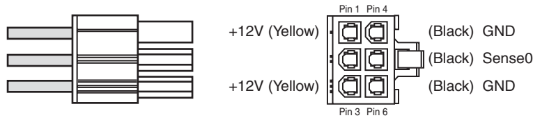
Figure 18.33 PCI Express 6-pin (2x3) auxiliary 75W power supply connector.
