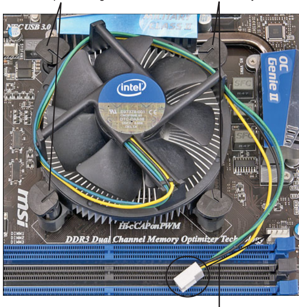
Figure 19.10 An Intel heatsink being installed on an LGA1155 processor.
