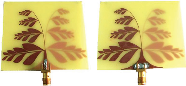
Figure 2.18 Prototype antenna. (a) Front view. (b) Back view.
