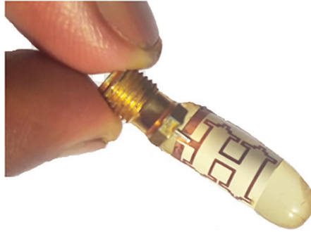
Figure 5.26 Fabricated antenna wrapped outside the capsule.
