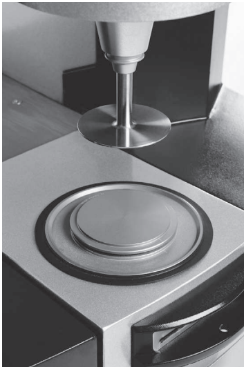
Fig. 1.9 A rotating parallel-disk rheometer (Image of Kinexus rheometer, used with kind permission of Malvern Instruments).
