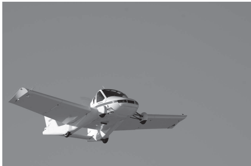
Fig. 7.30 The Transition ® car-plane in flight on March 23, 2012. It has a gross weight of 1,430 lbf and a cruise velocity of 105 mi/h. (Image from Terrafugia, Inc., http://www.terraflugia.com )
