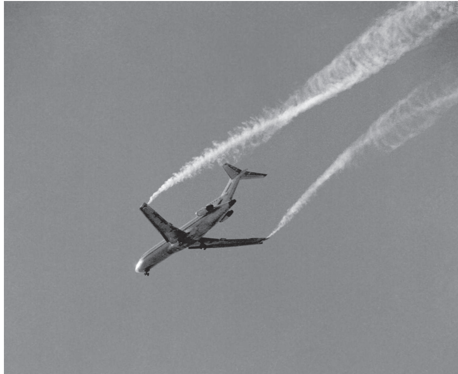
Fig. 8.27 Wingtip vortices from a smoke-visualization test of a Boeing 737. Vortices from large airplanes can be extremely dangerous to any following aircraft, especially small planes. This test was part of a research effort to alleviate these swirling wakes. ( NASA photo. )
