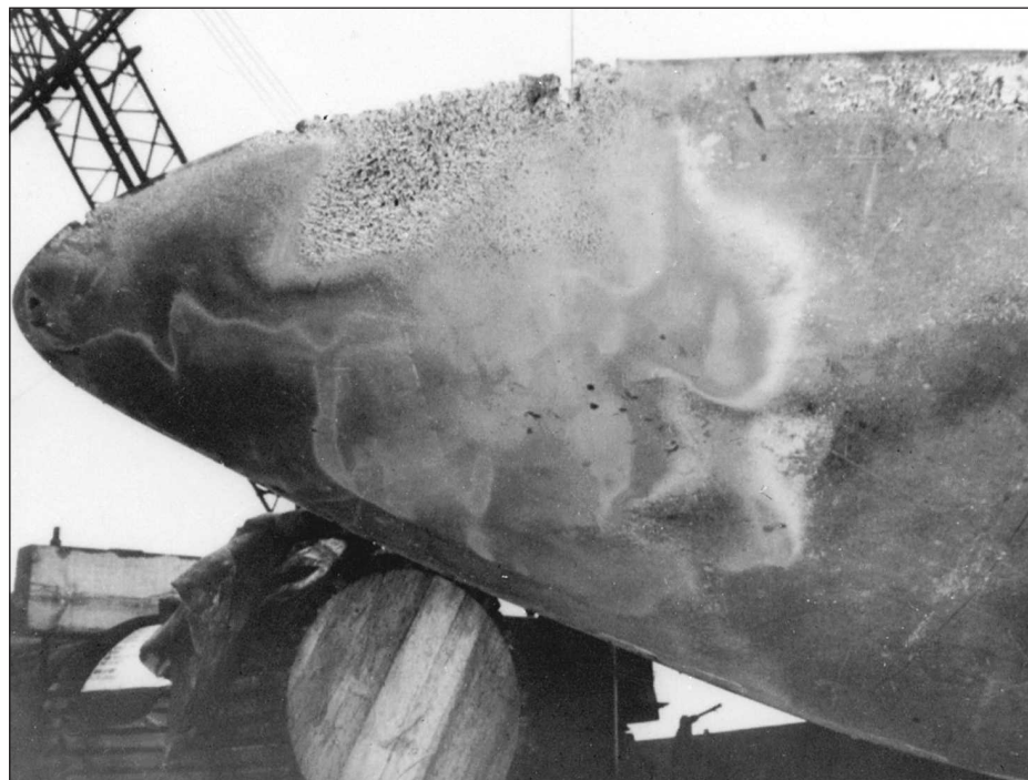
Fig. 1.14 Two aspects of cavitation bubble formation in liquid flows: (a) Beauty: spiral bubble sheets form from the surface of a marine propeller (courtesy of the Garfield Thomas Water Tunnel, Pennsylvania State University); (b) ugliness: collapsing bubbles erode a propeller surface (courtesy of Thomas T. Huang, David Taylor Research Center).
