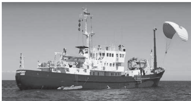
P7.85 Ship propulsion assisted by a large kite. (Courtesy of SkySails, Inc.)
