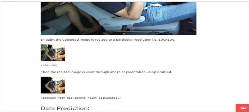
FIGURE 4.15 The pre-processed images, both resized and segmented, are updated as a part of the prediction process in the dashboard.
