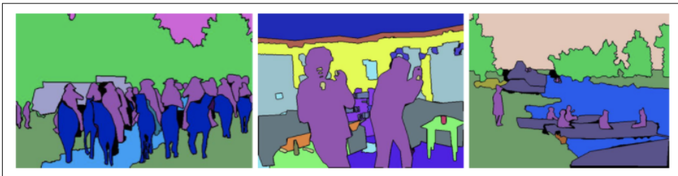
Figure 4-13. Image segmentation is a process of assigning a class to each pixel in an image. Here are some examples from the Common Objects in Context (COCO) dataset .
