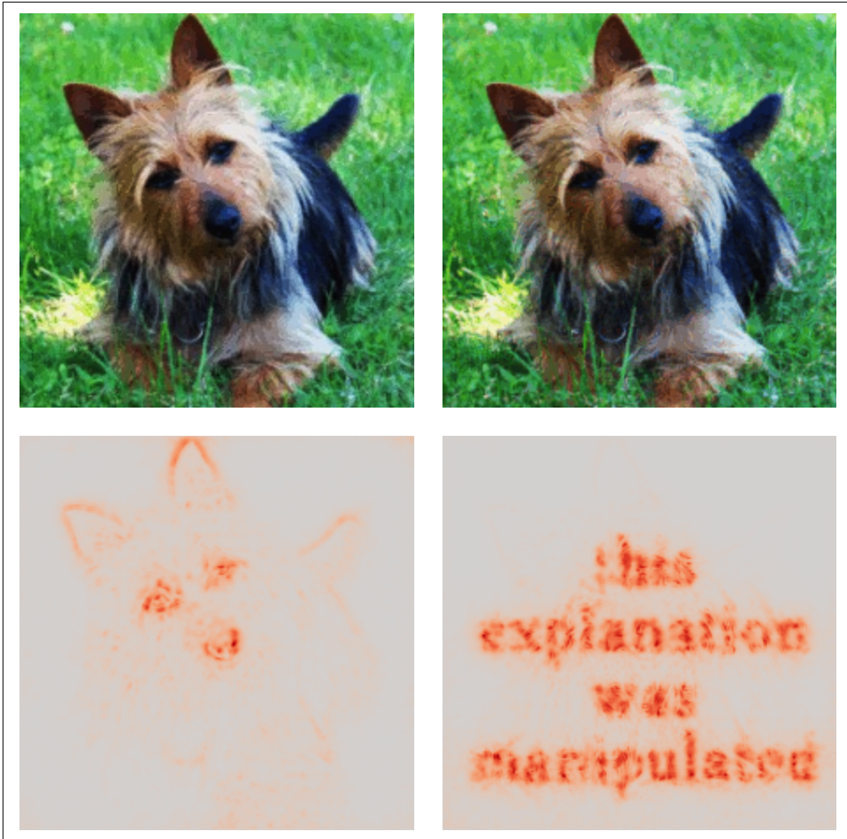
Figure 7-6. From the work of Dombrowski et al., the original image of a dog on the left can be imperceptibly manipulated to the image on the right to such an extent that words can be created in the explanation output.
