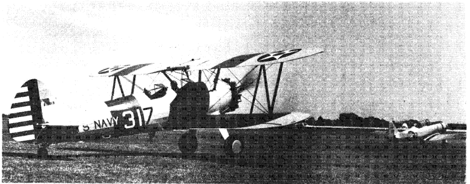
Figure 3-2 Shades of World War III! The trusty Stearman N2S—now an antique airplane capable of air show performance, aerobatics, crop dusting, and sport flying of any sort—but a demon when landing in severe crosswind conditions. An AT-6 is on right.
