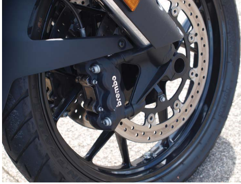
Figure 10.33 Radial brake mounting incorporated into fork end.
