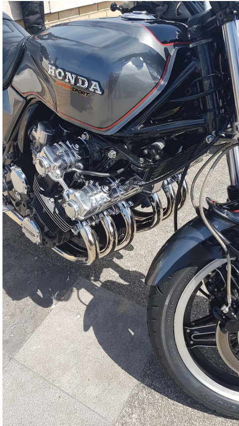
Figure 20.10 Six-cylinder exhaust pipes.
