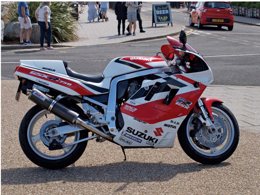
Figure 7.9 Classic Suzuki with aluminum semi-cruciform frame.
