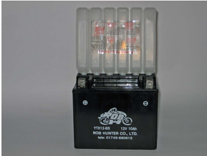
Figure 11.1 Battery being filled with electrolyte.
