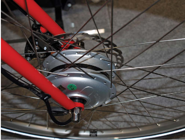
Figure 8.4 Electric bicycle with front-wheel mounted motor.
