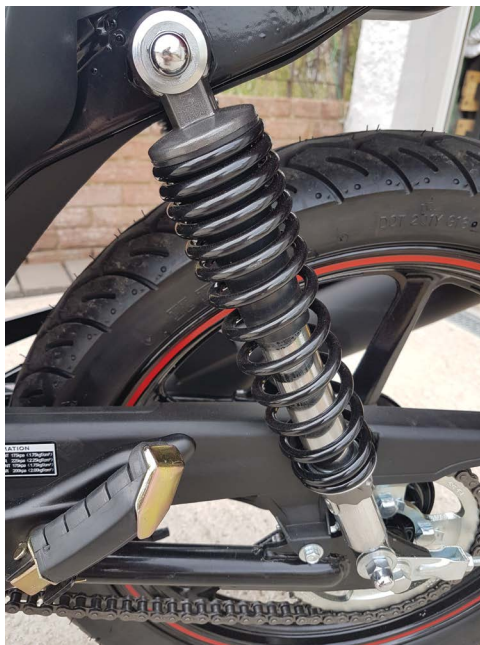
Figure 10.5 Lightweight coil over shock absorber.
