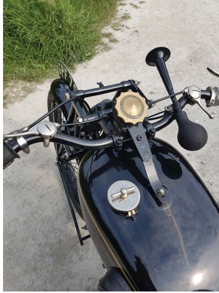
Figure 20.5 Cockpit of vintage motorcycle: left-hand side is clutch – obscured and advance and retard lever; center is brass knob for steering damper and bulb horn; right-hand side is choke lever and just visible end of front brake lever. On top of petrol tank is quick-lift, nondetachable filler cap.
