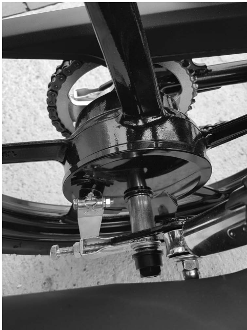
Figure 10.20 Drum brake on rear of lightweight 50 cc. You can see the adjustment nut.
