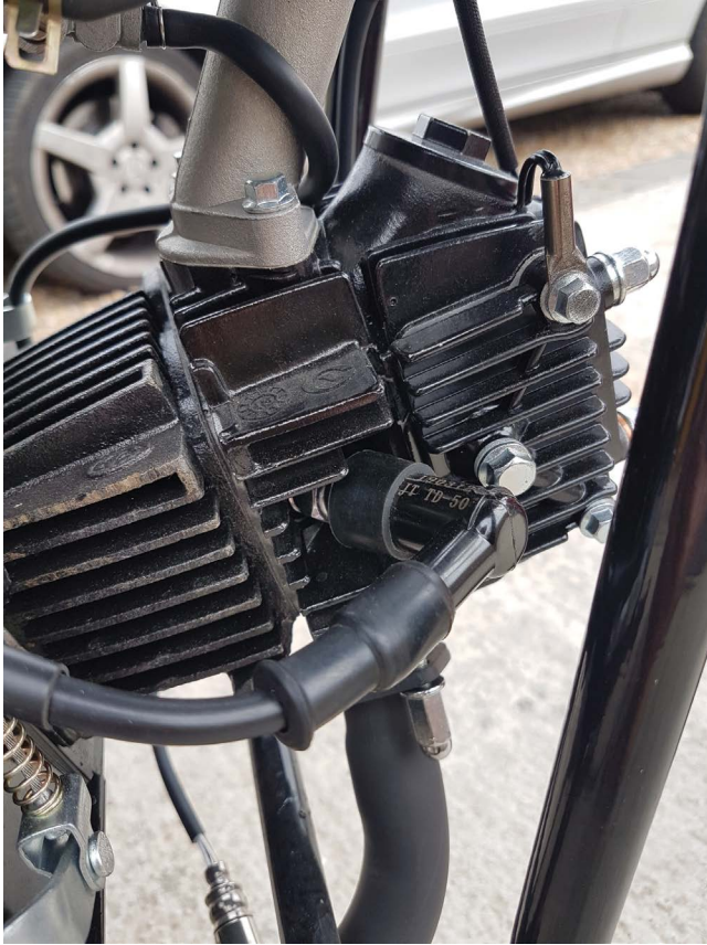
Figure 2.2 Spark plug in a single-cylinder 50-cc engine – it's a good idea to carry a spare spark plug and socket tool to change it in case of failure.
