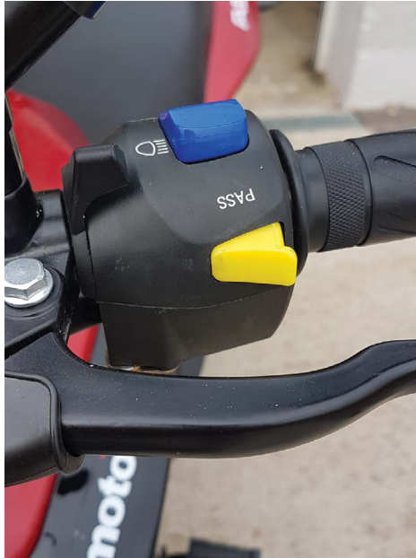
Figure 11.10 Yellow button is for pass-light.
