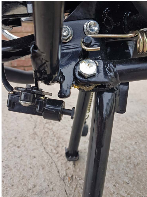
Figure 11.5 Switch to prevent riding off with the stand in the down position.
