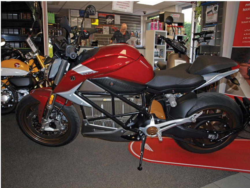
Figure 8.6 Zero electric motorcycle. The large gray part under what looks like the tank – which actually houses some of the electronics – is the battery. The orange/brown component is the electric motor; this directly drives the rear wheel with a belt.
