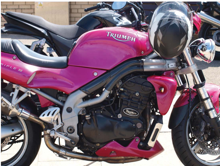
Figure 7.5 Classic Triumph twin-spare frame.
