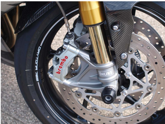
Figure 10.17 Crash bungs on fork ends and carbon fiber mud guards.
