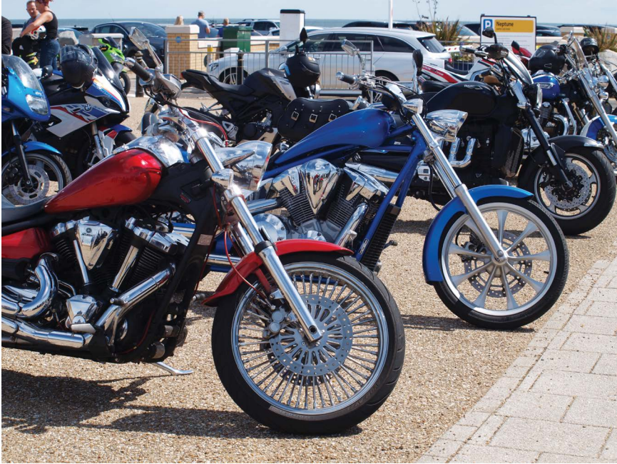
Figure 10.4 Large castor angles on these two cruisers.
