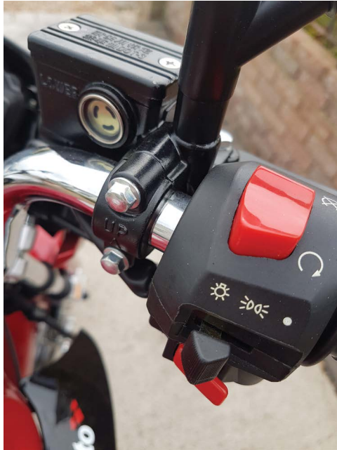
Figure 11.7 Top red rocker switch is emergency kill button, center is light switch, lower red is starter button.
