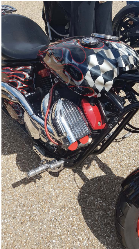
Figure 17.6 Slipped checkered pattern, CNC forward-mounted foot pegs, and drilled brake pedal.
