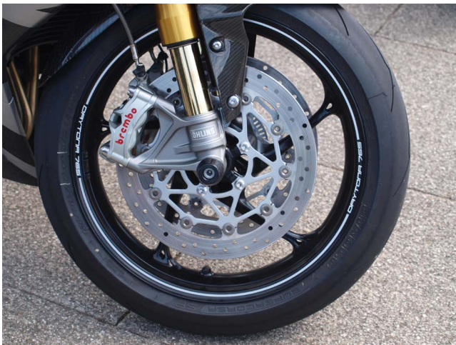
Figure 10.15 Dual disc radial brakes and upside-down forks.
