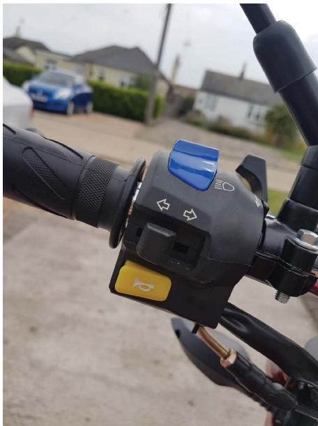
Figure 11.9 Blue switch on top is headlamp dip switch, black one in the middle is indicator switch, yellow push button is horn.
