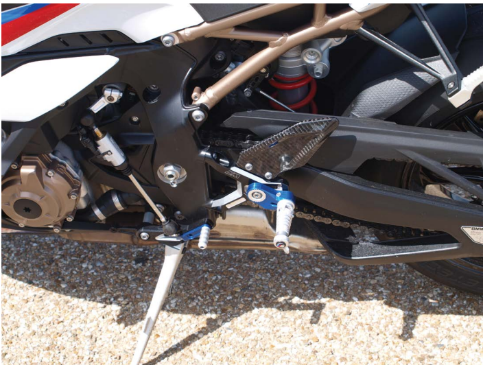
Figure 16.18 Nice carbon fiber plate to protect rider's boots from chain.
