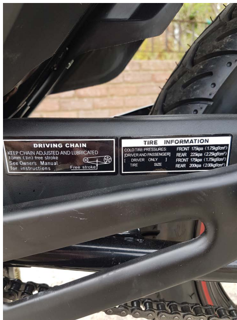
Figure 10.14 Tire pressure information sticker – found on most bikes.
