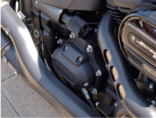
Figure 16.13 Separate gear box casing – nonunit construction.
