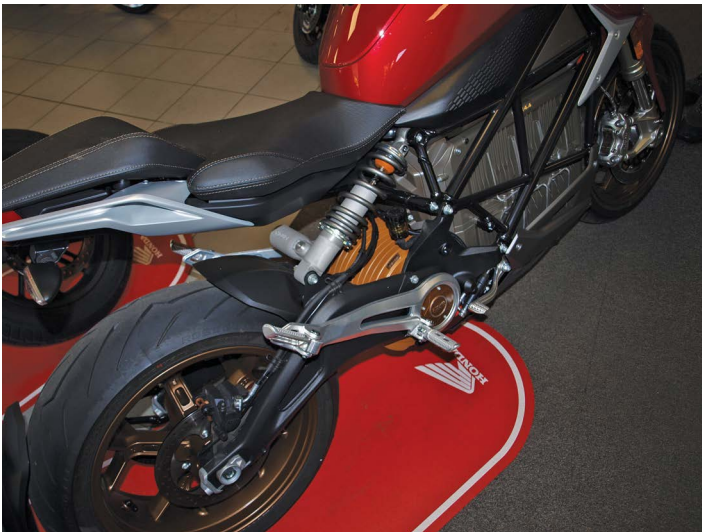
Figure 7.11 Rear view of Zero electric motorcycle. Note that the rear arm pivot is concentric with the motor shaft. The motor is the orange/brown part.
