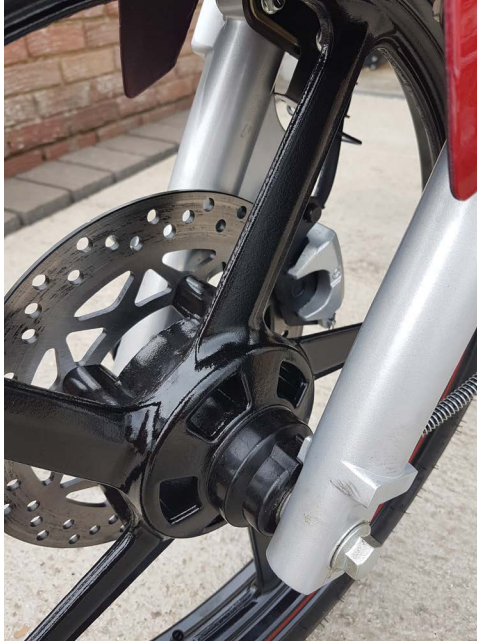
Figure 10.7 Lightweight wheel and single front disc.
