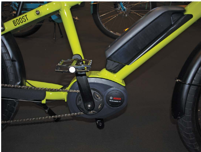
Figure 8.3 Electric bicycle with bottom-bracket mounted motor.
