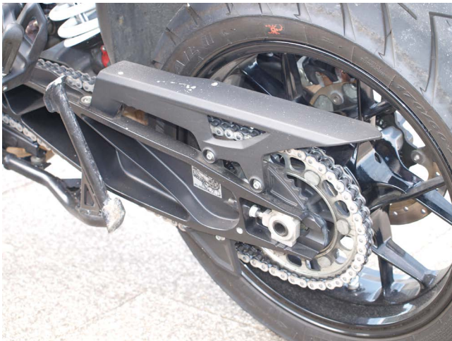
Figure 16.16 Chain adjuster on sports tourer motorcycle.
