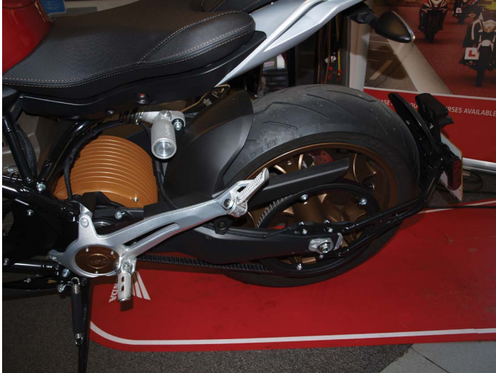
Figure 16.19 Toothed belt drive on a Zero Electric Motorcycle – similar to that used on Harley Davidson.
