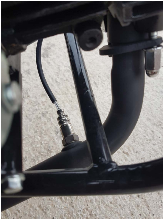
Figure 2.12 Lambda sensor to help control exhaust emissions.
