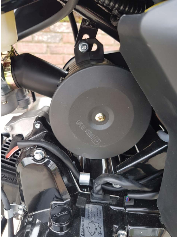
Figure 2.6 Air cleaner – you should check and clean this regularly.
