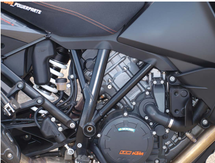
Figure 7.7 KTM with a mixture of cruciform and trellis.
