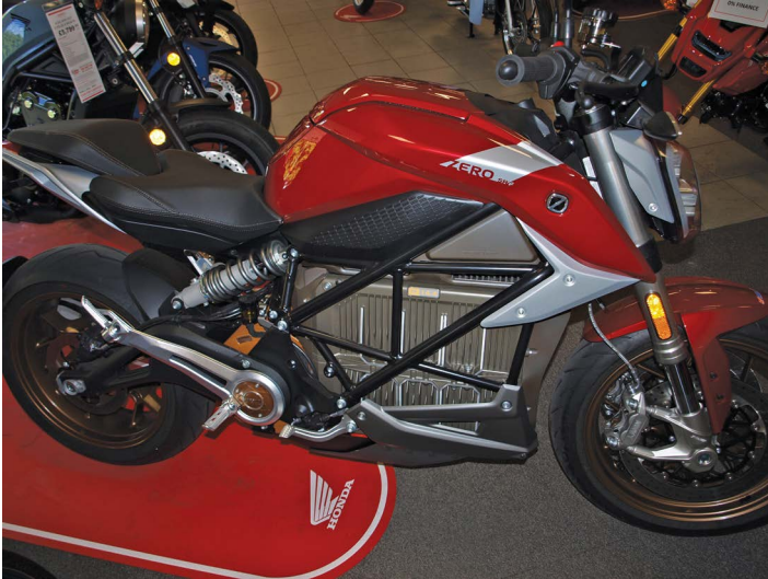
Figure 7.10 Zero electric motorcycle with heavy-duty trellis frame holding a battery box.
