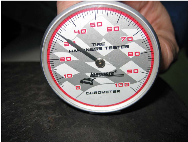
Figure 10.13 Durometer to measure tire hardness.
