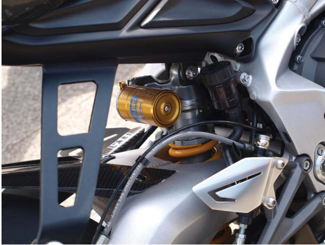
Figure 10.16 Heavy-duty rear adjustable shock absorber.
