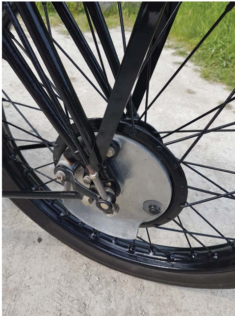
Figure 20.8 Vintage single-sided front drum brake.
