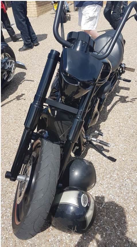
Figure 17.8 Hooded head lamp and shortened front guard, not to be used on rainy days.
