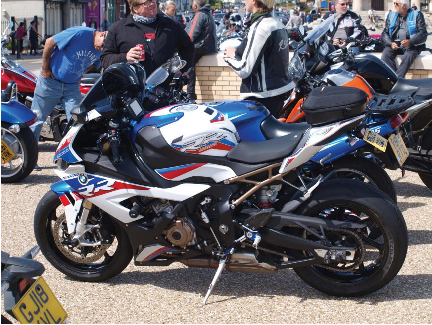
Figure 7.14 BMW S100 RR. Note crash bungs and position of prop stand.
