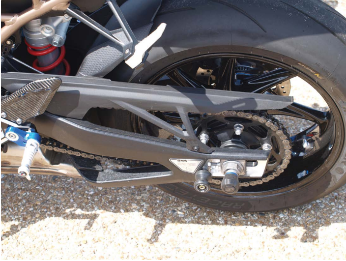
Figure 16.17 Notice crash bobbin on end of axle and bobbin for pit stand.
