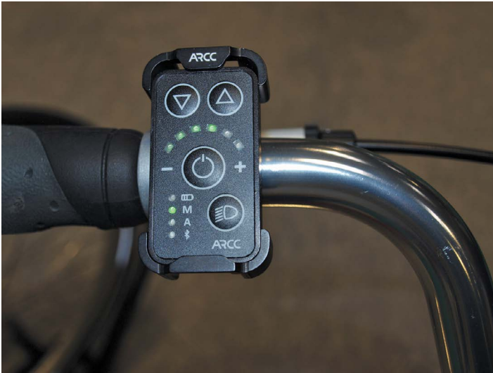
Figure 8.5 Control panel for electric bicycle.
