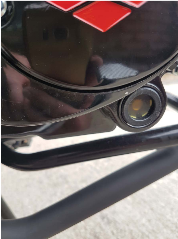
Figure 3.5 Sight glass to check oil level.
