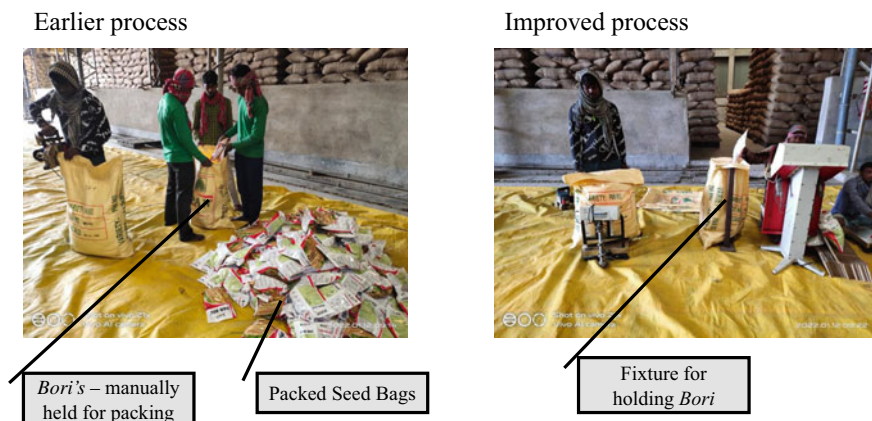
Fig. C1.8 Improvement in Bori filling
