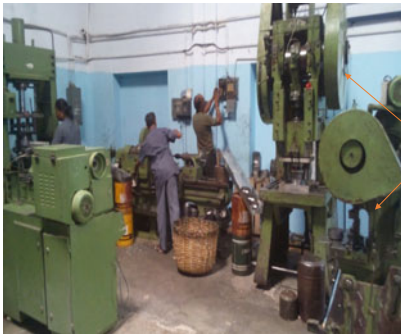
Fig. C7.8 Machine alignment to enable single worker operation
