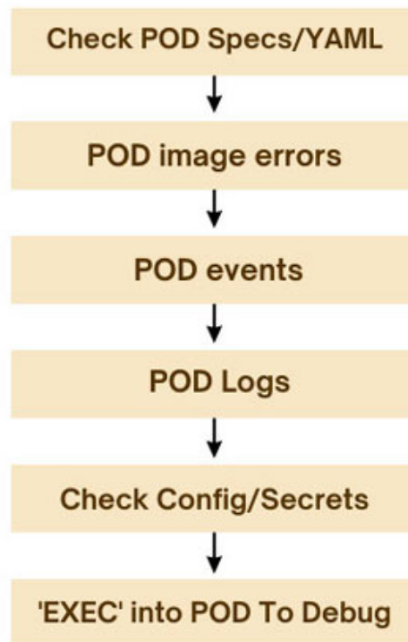
Figure 12.4: YAML syntax/validation->Pod image present->Pod events->Logs->ConfigMaps->Secrets->Storage Mounts-> exec into Pod
