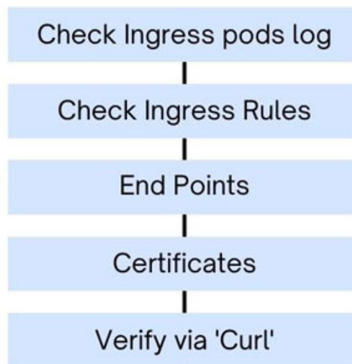
Figure 12.6: Ingress troubleshooting flowchart—get Ingress info, curl <ingress host>, check Ingress Pod, check certificate errors, verify via curl
