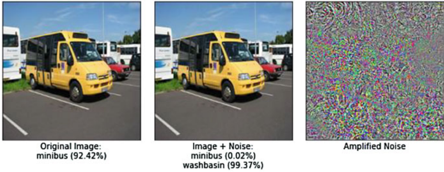
Fig. 7.2 An example of the result of the file-level privacy protection (the colors of noises are amplified by normalization otherwise they would be hard to see)
