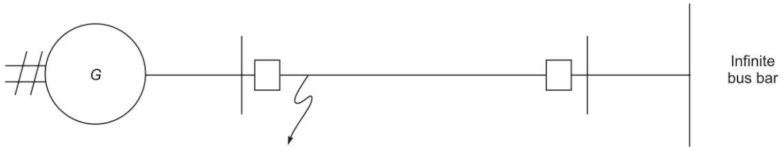
Fig. 8.53 A simple power system
