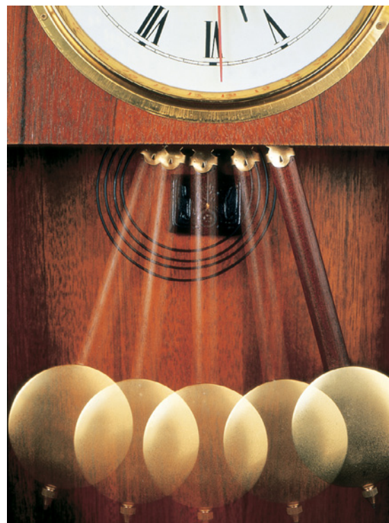
Fig. 9.1.3 The swinging pendulum controls the movement of the clock's hands. The pendulum is 0.248 m long, from pivot to center of mass/gravity, so each cycle takes 1 s to complete and advances the hands by 1 second.
