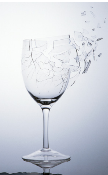
Fig. 9.2.6 Resonant energy transfer makes it possible for sound to shatter a crystal wineglass. When the sound pushes on the glass rhythmically, the sound slowly transfers energy to the glass, until it finally shatters. Because the sound must be extremely loud and at exactly the resonant frequency of the glass, only the most extraordinary opera singers can break a crystal wineglass.
