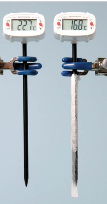
Fig. 7.2.3 You can determine the air's relative humidity using two thermometers, one of which has a wet cloth wrapped around its bulb (right). Evaporation cools the wet-bulb thermometer by an amount related to the air's relative humidity. The dryer the air, the colder the wet-bulb thermometer becomes.
