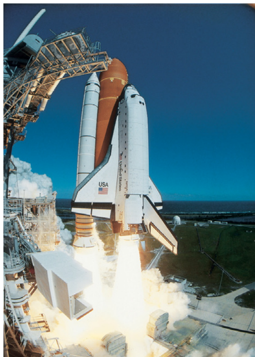
Fig. 4.2.3 The space shuttle's nozzles were designed to push its rocket exhaust downward as long glowing plumes. The gas pushed back, lifting the shuttle upward into space.
