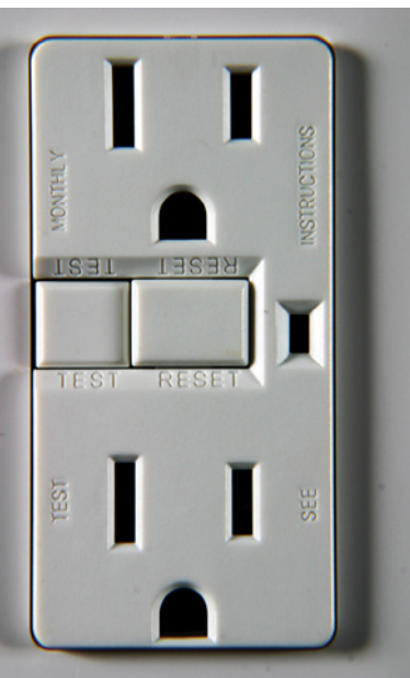
Fig. 11.2.2 This electric outlet follows the U.S. standard for 120-V AC, 15-A service. The wide slots (left) are neutral, the narrow slots (right) are hot, and the curved holes (center) are ground. This outlet provides ground-fault circuit interruption (GFCI) protection; if any current leaving hot fails to return to neutral, or vice versa, the outlet shuts off instantly until it is reset. The test button simulates a current leak and will shut off the outlet if its protection is functioning properly.
