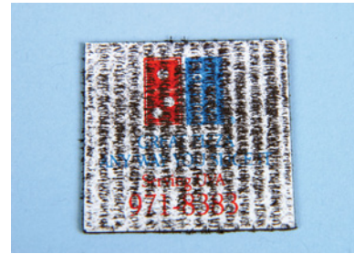
Fig. 11.1.5 Iron powder forms bridges between the magnetic poles of this plastic sheet magnet.
