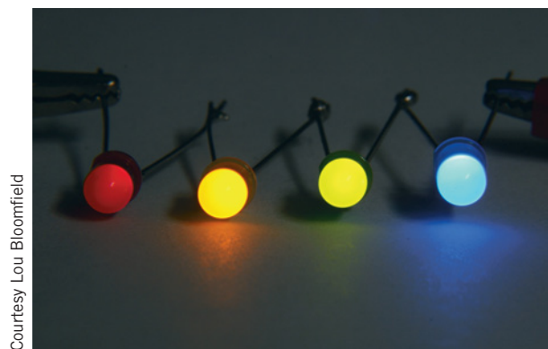
Fig. 13.3.8 These LEDs are connected in series so that the same current flows sequentially through each of them. However, their different band gaps cause them to emit different colors of light.
