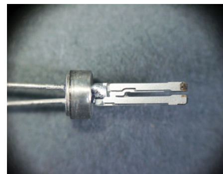
Fig. 9.1.10 Shaped like a tiny tuning fork, this watch crystal vibrates almost exactly 32,768 times per second. Burn marks at its tips were created when its vibrational frequency was tuned by a laser beam.
