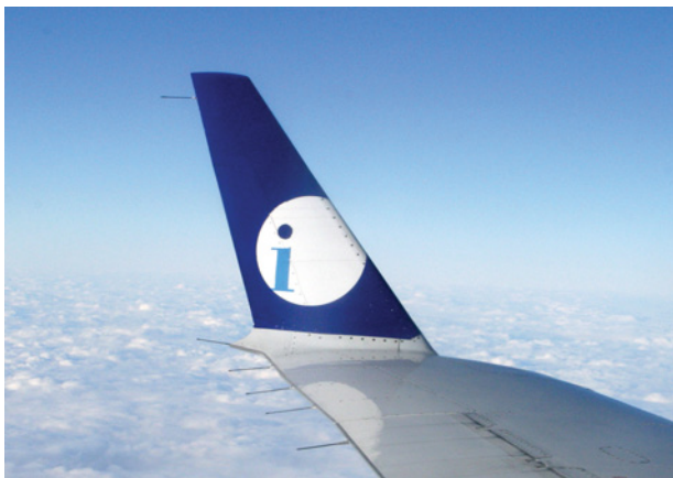
Fig. 6.3.7 This vertical wingtip keeps air from flowing around the end of the wing, a motion that would otherwise leave a powerful vortex in the air trailing behind the plane. Such wingtip vortices waste energy and are hazardous for other aircraft.
