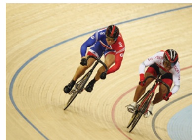
Fig. 4.1.7 As they round a turn during a race, these cyclists lean toward the inside of the turn. This leaning prevents the pavement from producing torques on them and tipping them over.
