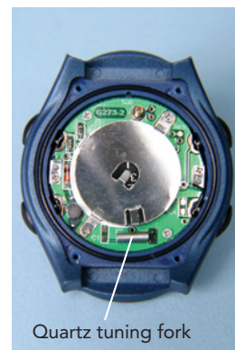
Fig. 9.1.9 The quartz crystal in this wristwatch is located inside the silver cylinder at the bottom. Carefully polished to vibrate at a precise frequency, the crystal keeps the watch accurate to a few seconds a month.
