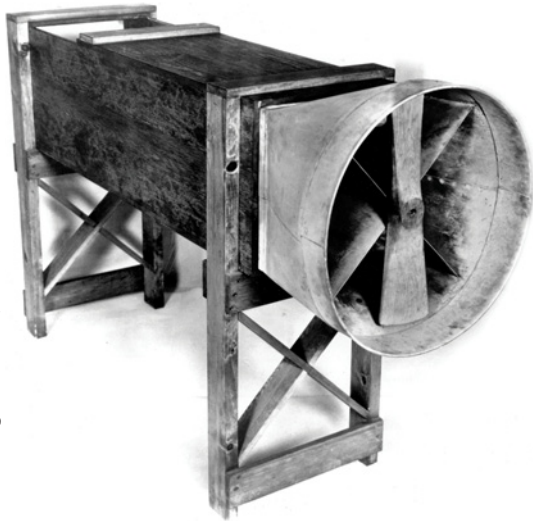
Fig. 6.3.10 The Wright brothers were accomplished aerodynamicists, using this wind tunnel to study and perfect wings and propellers for their airplanes.
