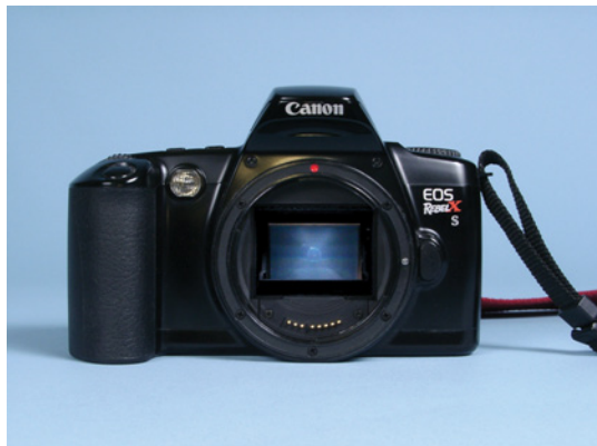
Fig. 14.1.10 The mirror in the center of this reflex camera directs light from the lens (removed for this photograph) onto the focusing screen above it. During the exposure, the mirror swings upward to permit light from the lens to strike the image sensor at the back of the camera.
