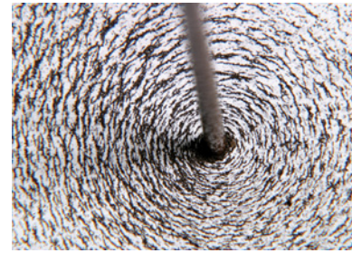
Fig. 11.1.9 Iron powder shows that flux lines around a current-carrying wire form concentric rings around that wire.
