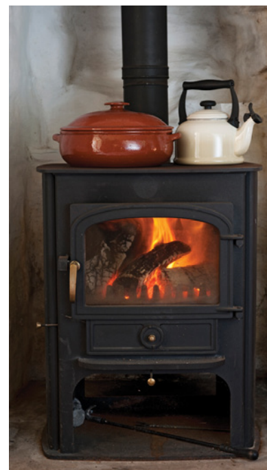
Fig. 7.1.1 This woodstove transfers heat to the room by conduction through its metal walls, convection of air past its surfaces, and radiation from its black exterior.
