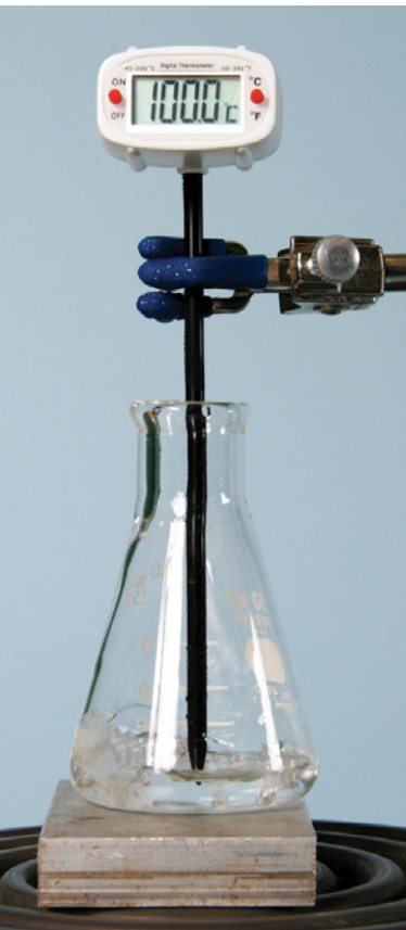
Fig. 7.2.4 Water boils at 100 °C, when atmospheric pressure can no longer smash the bubbles of water vapor.
