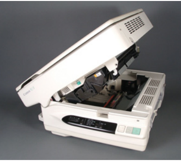
Fig. 10.2.4 This xerographic copier places the photoconductor drum, toner supply, and a corona wire inside a disposable cartridge. After the paper passes through the cartridge, toner is fused onto its surface and it leaves the copier.
