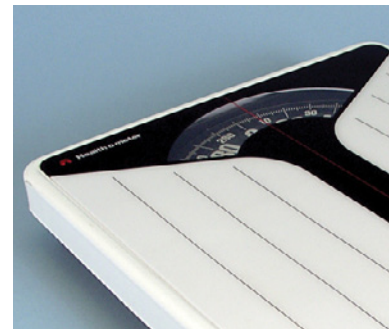
Fig. 3.1.4 When you step on this bathroom scale, its surface moves downward slightly and compresses a stiff spring. The extent of this compression is proportional to your weight, which is reported by the dial. Levers inside the scale make it insensitive to exactly where you stand.
