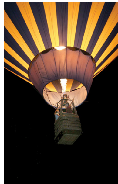
Fig. 5.1.5 The bottom of a hot-air balloon is open so that heated air can flow in and cold air can flow out. The heated air displaces more than its weight in cold air and makes the balloon lighter.
