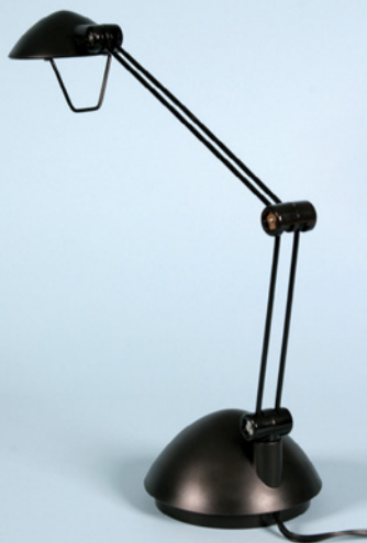
Fig. 11.2.7 The bulb in this halogen desk lamp operates from low voltages provided with the help of a transformer. The lamp's two support rods also carry 12-V AC current to and from the bulb.
