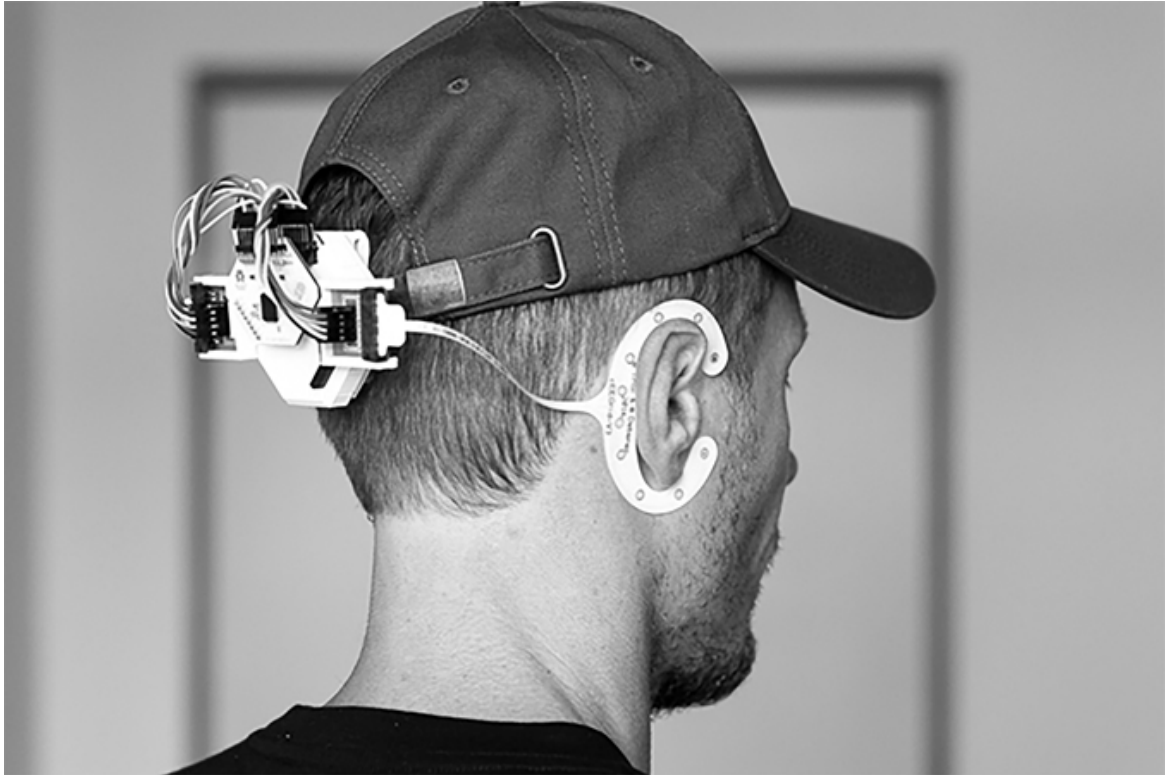
FIGURE 6.3 OpenBCI provides hardware for researchers interested in exploring Brain Computer Interfaces. ( Image Credit: OpenBCI.)
