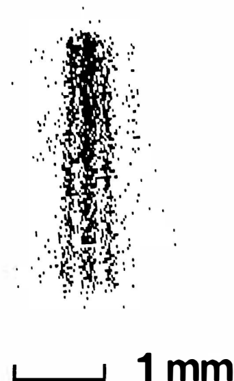
FIGURE 3. Observed Young's interference fringes of the metastable state neon atoms.
