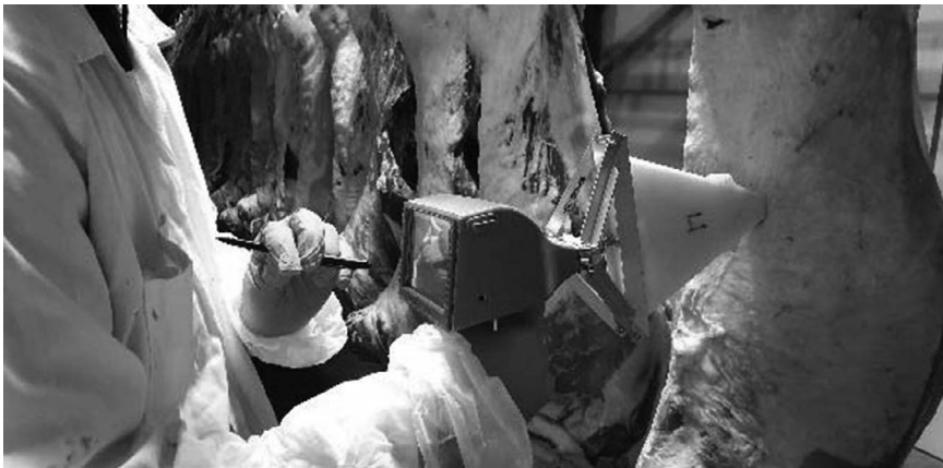
FIGURE 9.2 Measuring Carcass C-site Fat Depth using Microwave Device.
