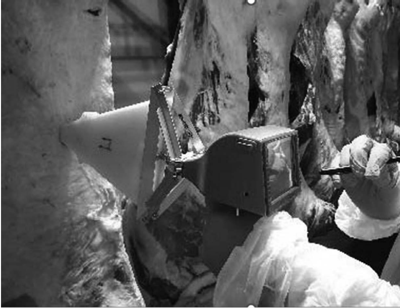
FIGURE 6.2 Measuring Carcase C-site fat depth using microwave device.
