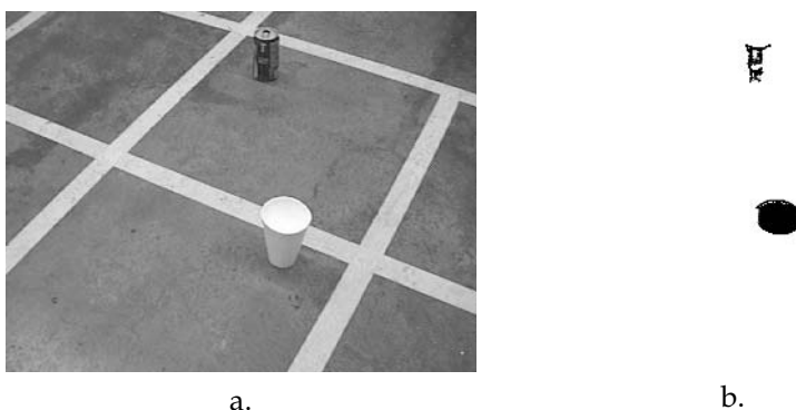
Figure 6.16 Segmentation of a red Coca Cola can: a.) original image and b.) resulting red regions. Note that some non-object pixels showed a reddish color.
