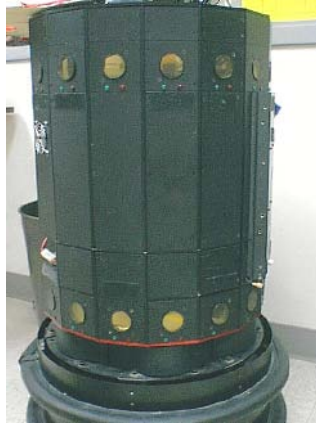
Figure 6.2 Example of redundant top and bottom sonar rings.
