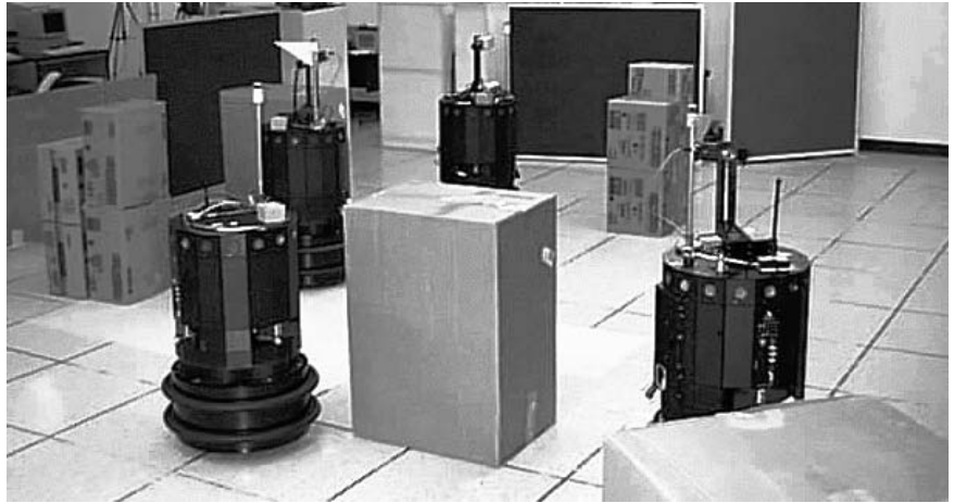
Figure 8.5 Robots cooperatively tracking an object under the ALLIANCE architecture. (Photograph courtesy of Oak Ridge National Laboratories.)
