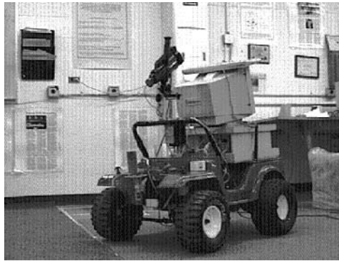
Figure 5.4 Omnibot, a mobile robot built from a Power Wheels battery-powered toy jeep by students and Omnitech Robotics, Inc.
