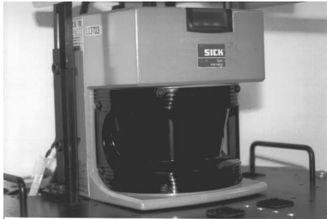
Figure 6.28 Sick laser, covering a 180° area.
