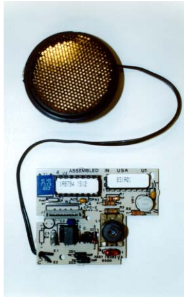
Figure 6.5 Polaroid ultrasonic transducer. The membrane is the disk.
