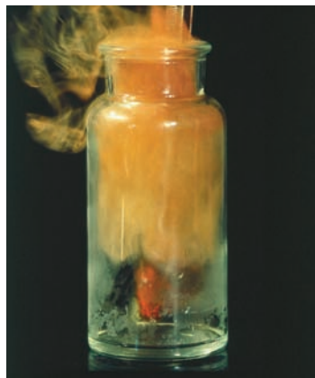
◀ Iron in Chlorine Gas Iron wool reacts in chlorine gas to give sparks and a yellow-brown \text{FeCl}_3 residue.
