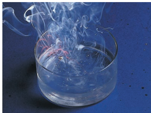
▲ Potassium in Water Potassium metal reacts violently in water as shown; potassium chloride, \text{KCl} , simply dissolves in water.
