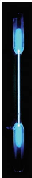
▲ Mercury Gas Discharge Tube The emission lines from mercury vapor illuminates the glass tube with a blue glow.
