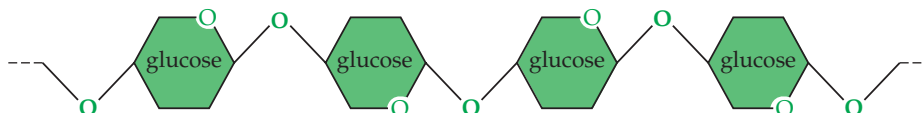
◀ Figure 20.12 A Segment of Cellulose Cellulose is a polymer of repeating glucose units. Note the position of the “O” in each glucose ring, which indicates that every other glucose unit is flipped upside down.
