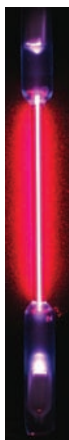
◀ Hydrogen Gas Discharge Tube The emission lines from hydrogen gas illuminate the glass tube with a reddish-purple glow.
