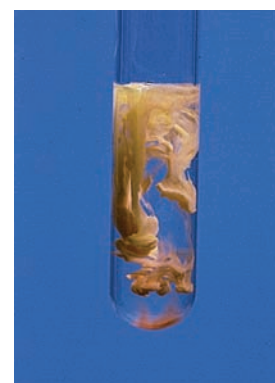
◀ Precipitation of \text{HgI}_2 Potassium iodide and mercury(II) nitrate react to give an orange precipitate of \text{HgI}_2 .
