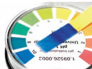
▲ pH Test Strip The indicator test strip paper uses universal indicator to test for pH. The test strip shown indicates a base at pH 10.
