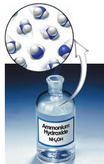
▲ Ammonia, \text{NH}_3 Aqueous ammonia, \text{NH}_3 , is found in laboratory reagent bottles labeled "ammonium hydroxide," \text{NH}_4\text{OH} .
