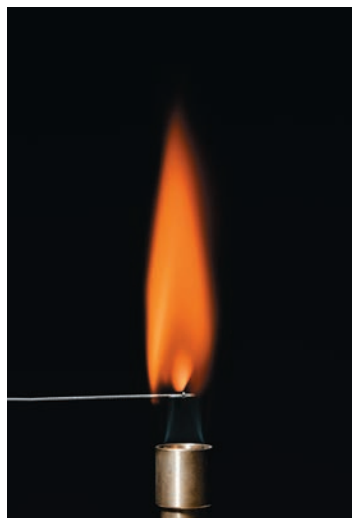
◀ Calcium Flame Test The flame test for calcium is red-orange.
