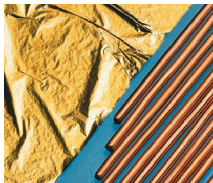
◀ Gold Foil and Copper Rods Gold and copper are both malleable and ductile metals; that is, each can be hammered into a foil and drawn into thin rods.
