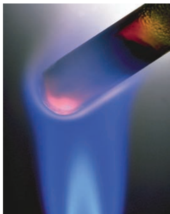
▲ Producing FeS Heating a mixture of iron powder and sulfur powder produces iron(II) sulfide; either the iron or the sulfur can be the limiting reactant.
