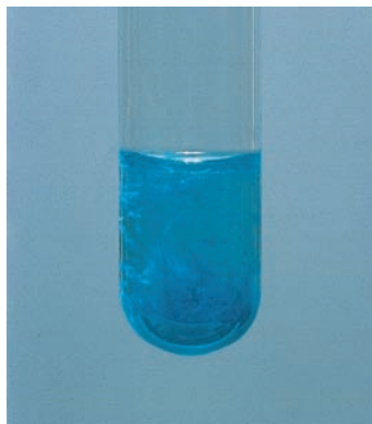
▲ Precipitate of \text{CuCO}_3 The aqueous solution reaction of \text{Cu}(\text{NO}_3)_2 and \text{Na}_2\text{CO}_3 yields a precipitate of \text{CuCO}_3 .
