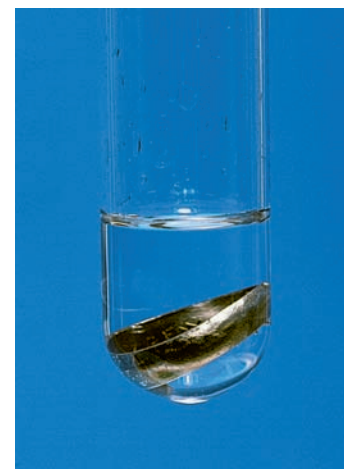
▲ Gold in Acid A gold ring gives no reaction in an aqueous sulfuric acid, \text{H}_2\text{SO}_4 , solution.
