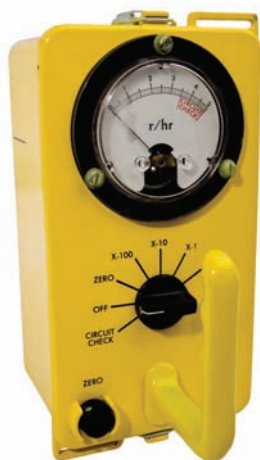
▲ Figure 18.3 Geiger Counter A Geiger counter gives a “click” each time a radioactive nucleus decays and releases a particle.
