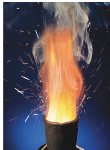
▲ Thermite Reaction The thermite reaction of iron oxide and aluminum metal produces molten iron and a shower of sparks.
