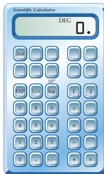
▲ Scientific Calculator A scientific calculator has an exponent key (EXP) for expressing powers of 10.
