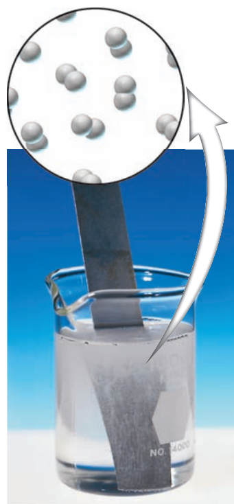
◀ Magnesium in Acid Magnesium metal reacts in aqueous sulfuric acid, \text{H}_2\text{SO}_4 , to give bubbles of hydrogen gas.
