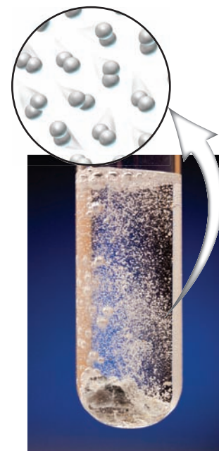
▲ Calcium in Water A piece of calcium metal in water reacts to give bubbles of hydrogen gas.
