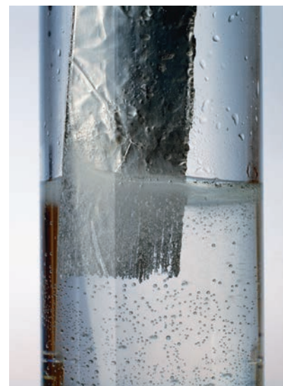
▶ FIGURE 14.2 Acids dissolve many metals When aluminum is put into hydrochloric acid, the aluminum dissolves. QUESTION: What happens to the aluminum atoms? Where do they go?
