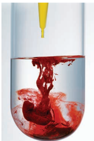
▲ FIGURE 7.3 A precipitation reaction The formation of a solid in a previously clear solution is evidence of a chemical reaction.
