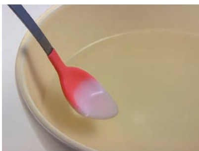
▲ A child's temperature-sensitive spoon changes color upon warming due to a reaction induced by the higher temperature.
