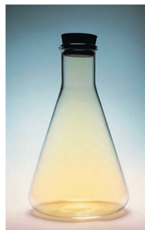
▲ FIGURE 5.2 Elemental chlorine Chlorine is a yellow gas with a pungent odor. It is highly reactive and poisonous.
