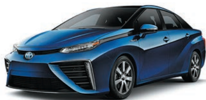
▲ FIGURE 16.1 A fuel-cell car The Toyota Mirai is the first mass-produced fuel-cell vehicle. It is powered by hydrogen and its only emission is water.
