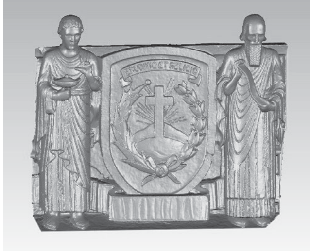
Figure 7.11 Processed and aligned scan data of shield as seen within the modeling software
