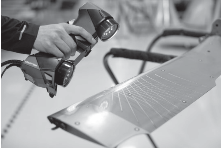
Figure 3.10 Tethered unit with laser grid lines on propeller blade. Note small circular black and white dots to enable tracking of the scanner
