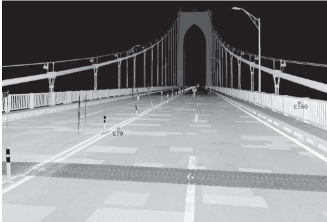
Figure 7.20 View of scan data showing level of detail captured on road surface
