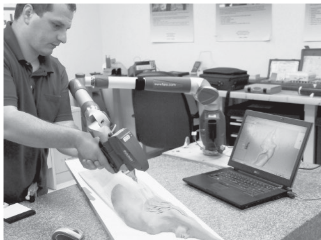
Figure 6.17 Scanning technician using an arm scanner to record the surface of the artist's sculpture
