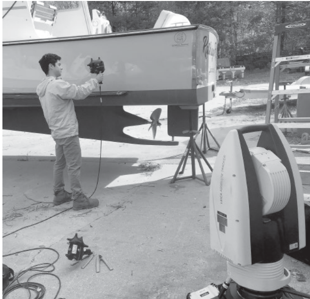
Figure 3.12 Handheld laser scanner/laser tracker system being used to scan boat hull
