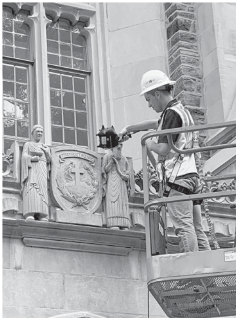
Figure 7.10 Use of a handheld scanner to record intricate detail of ornamental objects
