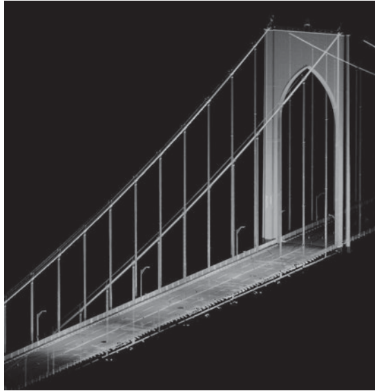
Figure 7.21 A view of multiple point cloud scans showing a portion of the bridge. Nighttime scanning provided excellent return of laser light points, yielding dense high-quality data
