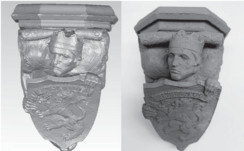
Figure 7.12 Completed dataset of scanned object with resulting 3D printed reproduction of the object
