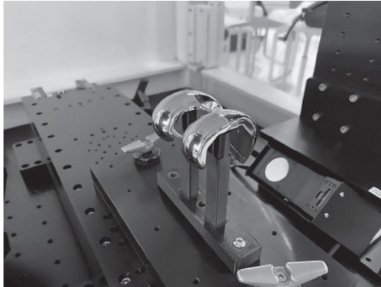
Figure 8.4 Prosthetic knee in 3D scanning device Source: Photo Courtesy of DWFritz Automation, LLC.
