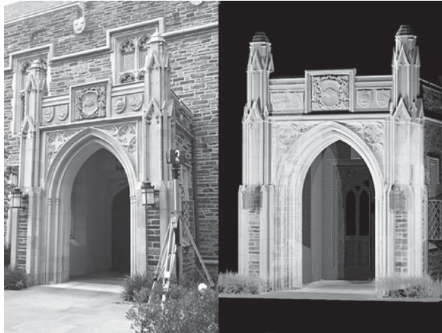
Figure 7.9 Tripod-mounted scanner and resulting scan data of building entry
