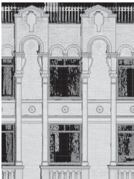
Figure 7.2 Note level of detail within the point cloud data, allowing for CAD delineation of façade elements
