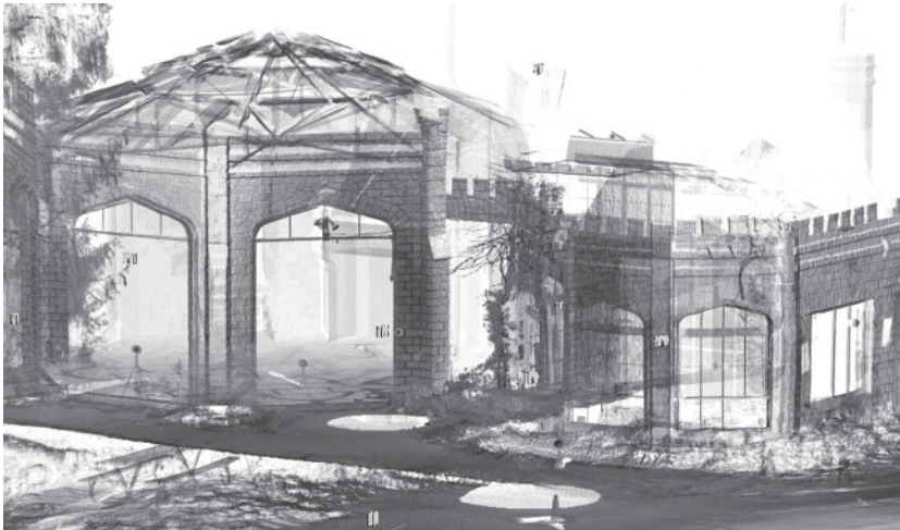
Figure 4.1 3D Point cloud data from multiple aligned scans as viewed within a processing software
