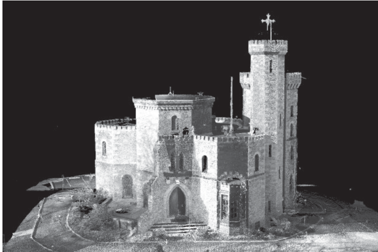
Figure 7.15 Multiple scans combine to form point cloud view of building within scan processing software
