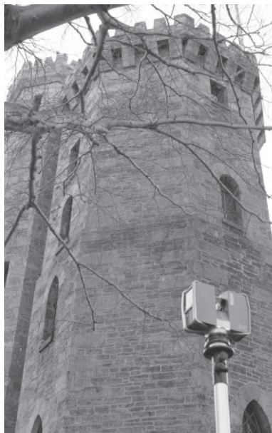
Figure 7.14 Use of an extension tripod allowed for better capture of data at upper levels
