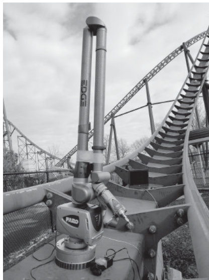
Figure 6.15 Sections of steel supports scanned at high resolution by the FARO arm scanner
