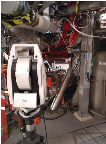
Figure 7.7 Laser tracker set outside the tokamak
