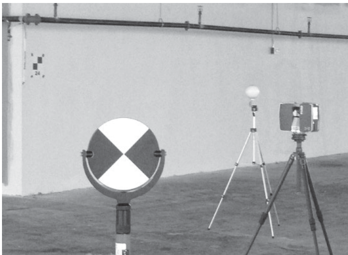
Figure 4.6 A LIDAR scanner with three common targets used when scanning on-site: A swivel-mounted checkerboard monopod for control points, a wall-mounted paper checkerboard target, and a target sphere
