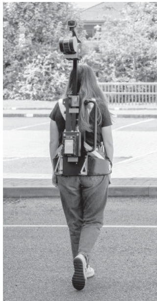
Figure 3.16 Typical wearable SLAM device self-contained within a backpack assembly, designed to capture point cloud data as one walks through a space Source: Image courtesy of GeoSLAM, www.geoslam.com .
