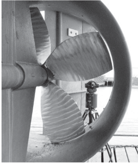
Figure 6.12 The laser tracker set in place scanning the propeller
