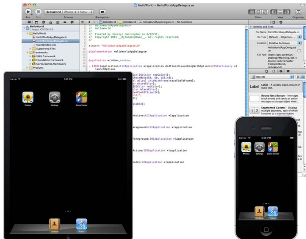
Figure 1.3 The SDK includes Xcode (top) and two instances of the iOS Simulator, running in iPad mode (bottom left) and iPhone mode (right).
