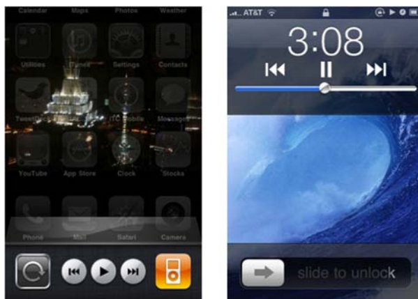
Figure 22.4 Two remote-control UIs on the iPhone when the audio application is playing in the background
