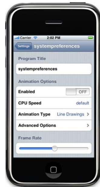
Figure 8.4 As seen on an iPhone, in order from top to bottom, a Group , a TextField , another Group , a Switch , a TitleValue , a MultiValue , a ChildPane , a third Group , and a Slider
