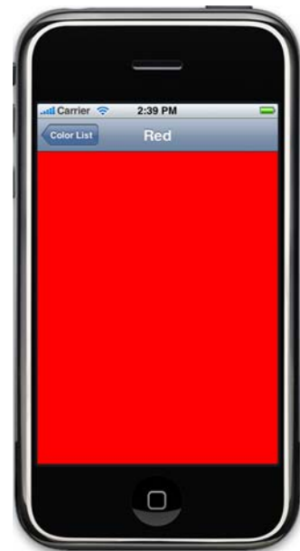
Figure 7.7 With a few simple commands, a navigation controller's setup is largely automated. Here you see the titled navigation bar with a titled back button.
