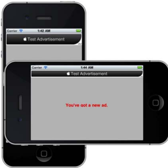
Figure 20.4 Dynamically update the banner view size to support both portrait mode and landscape mode.
