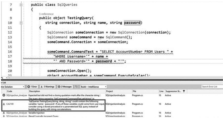
FIGURE 14.9 The code analysis results of the code analysis feature on Visual Studio Enterprise indicates the risk of SQL injection caused by flaws in the source code.
