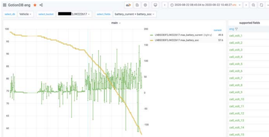
Figure 7.3 A typical dashboard for displaying battery data, developed by Gotion [6].
