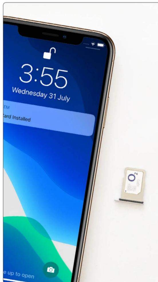
**2** Use a SIM eject tool like the one pictured here, or maybe a straightened paper clip, and insert it into the small hole next to the SIM slot. The tray then pops out as shown.
