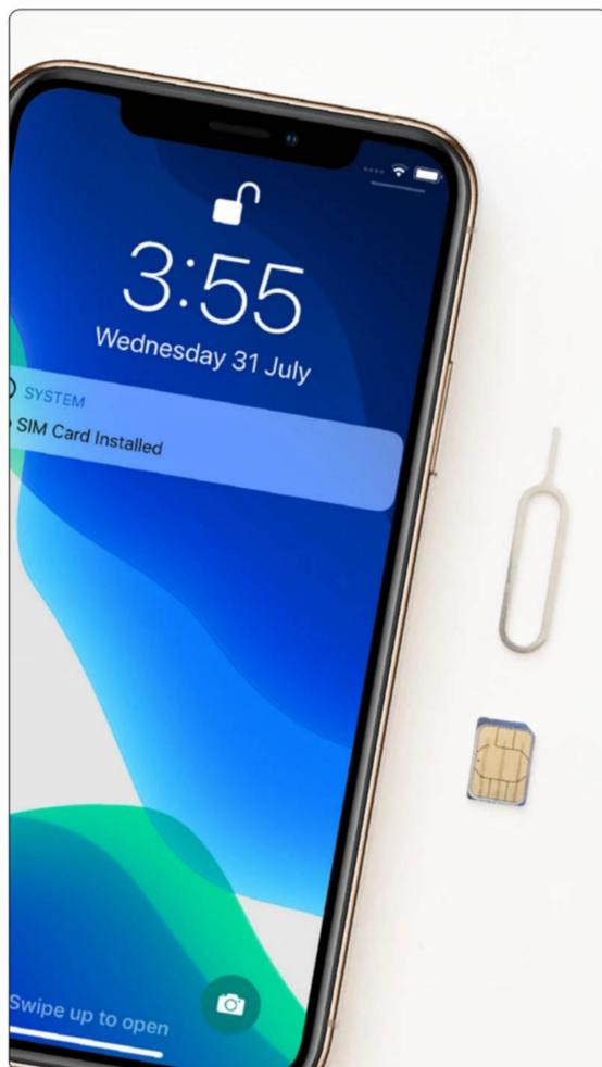
**1** To activate your iPhone, you must first insert the Nano-SIM card provided by your mobile phone network provider. An eSIM card is non-removal as detailed below.
