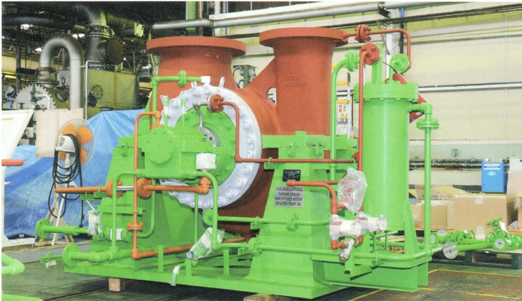
FIG. A1.19 Photo of thermal-power-plant-boiler feedwater booster pump. Courtesy and copyright of MHI
