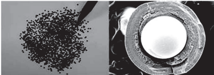
Figure 13.16. KAERI's pilot TRISO fuel particles and a microscopic image
