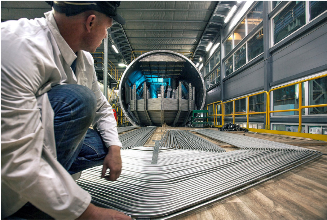
FIG. A1.64 Heat-transfer tubes for steam generator (ПГБ-1000) for VVER-1200 (Generation-III + ), 1110 MW el , Unit 2, Belarus' NPP (2 units in operation). Courtesy of Rosatom: https://www.flickr.com/photos/rosatom/36999718643/in/album-72157675727427445/ ; Photo by E. Lyadov, Atommash, 2016
