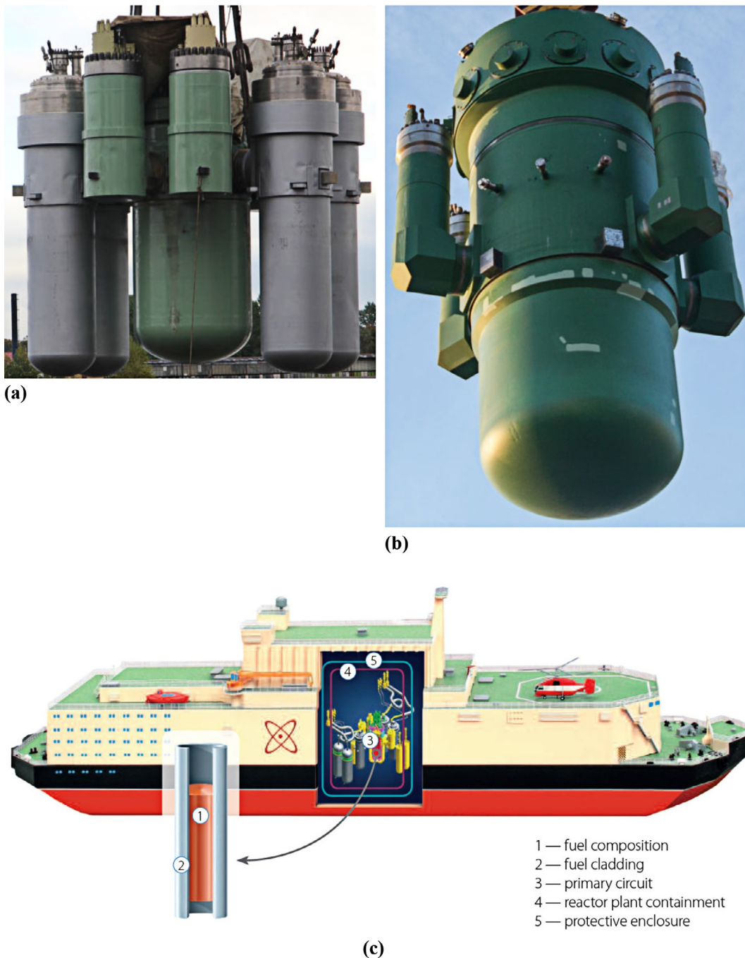
FIG. A1.66 Photos of Russian SMRs – PWRs: (a) KLT-40S (Generation-III): large grey cylinders – 4 steam generators and small green cylinders – 4 circulation pumps. Two reactors installed on a barge and operate as floating NPP (Port Pevek). (b) Generation III + SMR - RITM-200M with steam generators integrated into pressure vessel; small cylinders – circulation pumps. NPP with these reactors will be built in Yakutia. (c) Defense-in-depth arrangement schematics of floating NPP Courtesy of Rosatom. (a) Photo Baltzavod, 2013: https://www.flickr.com/photos/rosatom/42425233062/in/album-72157692330711570/ and (b) Photo by N. Greidin, Baltzavod: https://www.flickr.com/photos/rosatom/24835999197/in/album-72157671934046766/ ; and (c) Courtesy of JSC “Afrikantov OKBM”, Nizhny Novgorod, Russia: http://www.okbm.nnov.ru/upload/iblock/69e/40i3dob8nyjigsaoe5tlunlij2qr2mh9.pdf ; accessed Feb. 19, 2022
