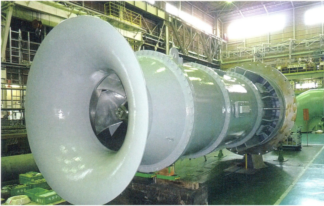
FIG. A1.17 Photo of thermal-power-plant water-circulating pump. Courtesy and copyright of MHI
