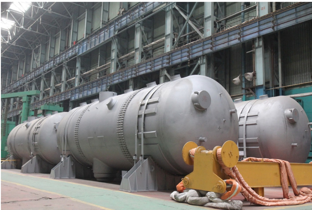
FIG. A1.63 Set of 4 steam generators (PIGB-1000) for VVER-1200 (Generation-III + ), 1110 MW el , Belarus' NPP (2 units in operation). Courtesy of Rosatom: https://www.flickr.com/photos/rosatom/37621538806/in/album-72157675727427445/ ; Photo by E. Lyadov, Atommash, 2017
