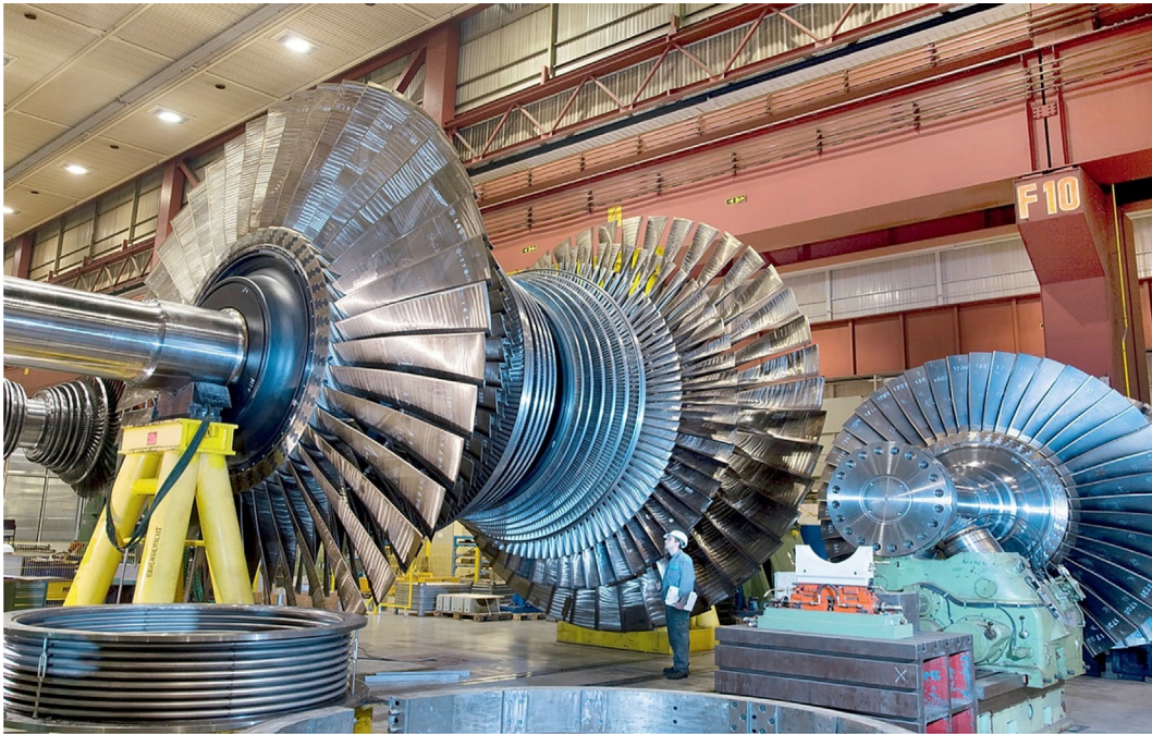
FIG. A1.5 Photo of Low-Pressure (LP) double-flow steam-turbine rotor with blades for supercritical-pressure coal-fired power plant. Siemens press photo; courtesy and copyright Siemens AG, Munich/Berlin, Germany
