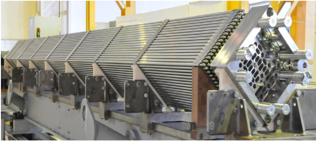
FIG. A1.54 Square-shape fuel bundle or assembly for PWRs (non-VVER type, also, see Fig. A1.44). Courtesy of Rosatom: https://www.flickr.com/photos/rosatom/33012084356/in/album-72157677073459854/ ; Photo by NZHK, 2009
