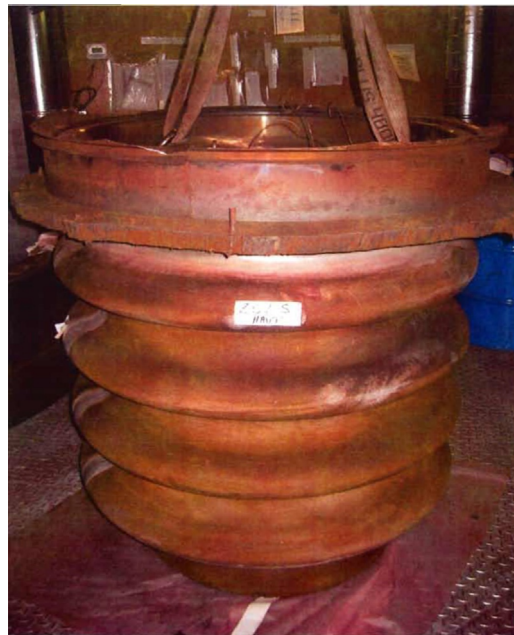
Figure 11.26. View of bellow tested on Superphenix heat exchanger (EFR Associates, 1998)
