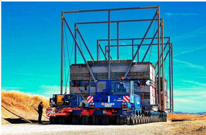
Figure 23.14. A 352-wheel platform, unique in Europe, is used to transport ITER’s highly exceptional loads from the Mediterranean Sea to Cadarache. Credit: ITER Organization
