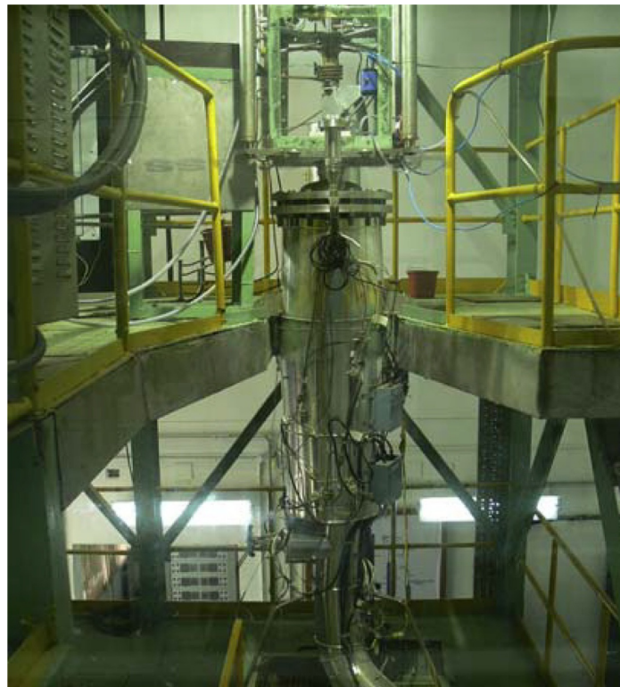
Figure 15.22. Sodium-Fuel Interaction Facility (SOFI): facility for molten fuel interaction studies
