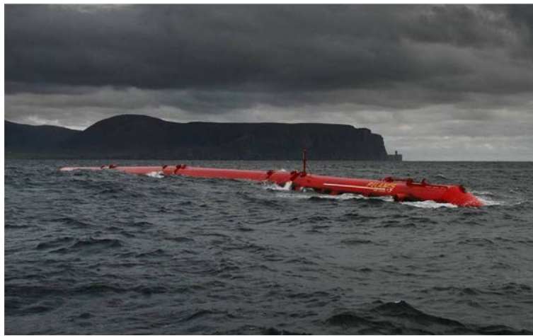
Figure 1.1.46. Photo of the Pelamis Wave-Energy Converter on site at the European Marine Energy Test Centre (EMEC), Orkney, Scotland, 2007. This converter was rated at 750kW and was the world's first off-shore wave-power machine to generate electricity into a grid system. The prototype is 120-m long and 3.5 m in diameter. It consisted of four tube sections linked by three, shorter, power-conversion modules. Photo taken from Wikimedia Commons, author/username P123. Source: Wikipedia
