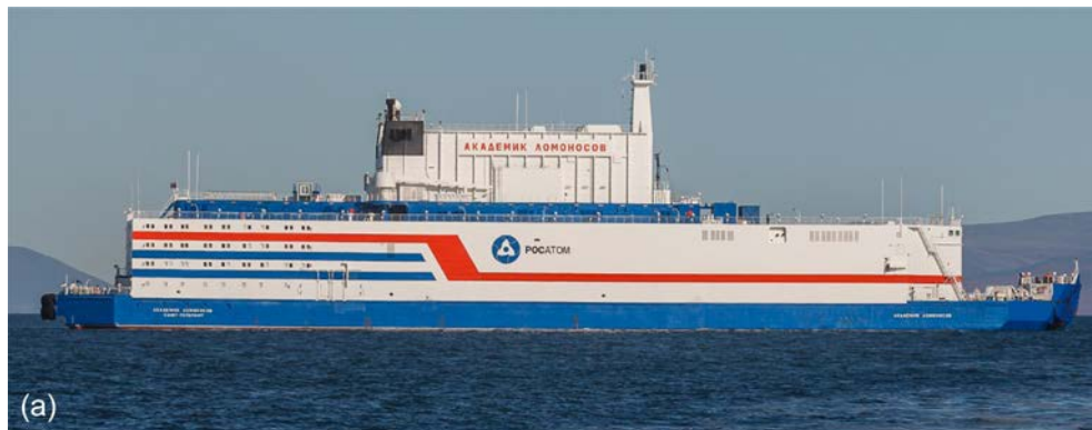
Figure 20.2.8. (a) Photo of Floating Nuclear Thermal-Power Plant (FNTThPP) (Плавающая Атомная Тепловая ЭлектроСтанция (ПАТЭС) (in Russian abbreviations)) on barge with two KLT-40S reactors on its way to port Pevek ( https://www.flickr.com/photos/rosatom/albums/72157692330711570 ; accessed Feb. 19, 2022). Barge: Length—140 m; width—30 m; height of board—10 m; draught—5.6 m; displacement—~21,000 t; underwater foundation pit in m—175 (L) × 45 (W) × 9 (D); operating term of FNTThPP—40 years; number of servicing personal—~70; and construction term—4 years.
