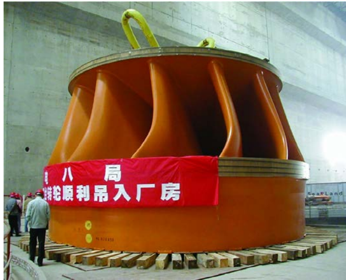
Figure 1.1.16c. Francis-turbine runner (Yangtze River, China). The Francis turbine is a type of water turbine developed by James B. Francis in 1848 in Lowell, Massachusetts. It is a high-efficiency (90% and beyond) inward-flow reaction turbine that combines radial and axial flow concepts. Francis turbines are the most common water turbine in use today. These turbines are primarily used for electrical-power generation and operate within the head range of 10 to 650 m and the power-output range of 10 to 750 MW el . In general, mini-hydro installations may be with even lower output power. Runner diameter can be between 1 and 10 m, and the speed range of turbine—from 83 to 1000 rpm. Large- and medium-size Francis turbines are most often arranged with a vertical shaft. However, small-size turbines have usually a horizontal shaft. Courtesy of Chinese National Committee on Large Dams. Source: Wikipedia
