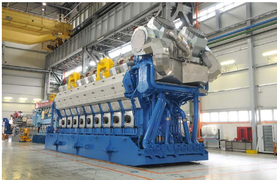
Figure 1.1.14. The largest in the world 18-cylinder Otto-cycle natural-gas-engine (18V50SG) power-generating unit with output of up to 18.3 MW el (~25,000 hp), 50 Hz and 500 rpm. The natural gas fueled, lean-burn, medium-speed engine is a reliable, high-efficiency and low-pollution power source for flexible base load, intermediate peaking and combined-cycle power plants. Efficiency—48.6%. Dimensions in m: length—18.8; width—5.33; height—6.34; bore—500 mm; and weight—360 t. Engine is 4-stroke spark-ignition with a prechamber. Courtesy of WÄRTSILÄ, Finland
