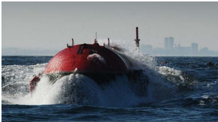
Figure 1.1.45. Photo of the first in the world 2.25-MW el Aguçadoura wave power plant (Portugal). Pelamis machine is made up of connected sections, which flex and bend relative to one another as waves run along the structure. This motion is resisted by hydraulic rams, which pump high-pressure oil through hydraulic motors, which in turn drive electrical generators. Three machines within three 120-m long cylinders, each rated at a peak output of 750 kW el , have been installed. The total peak power of 2.25 MW el enough to cover electrical needs of more than 1500 Portuguese homes. However, the average output from a Pelamis machine depends on the wave resource in a particular area. According to information on the Pelamis website, it appears that the average power output for a Pelamis wave machine is about 150 kW. Photo taken from Wikimedia Commons, author/username P123. Source: Wikipedia
