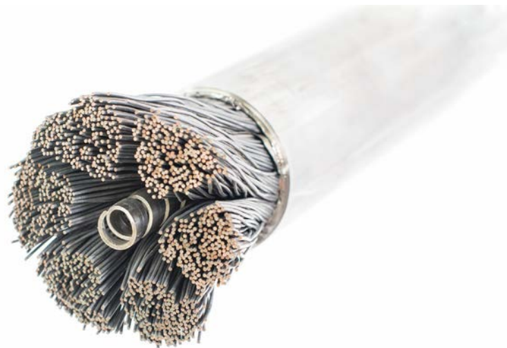
Figure 23.8. A section of a niobium-tin superconducting Cable-In-Conduit Conductor (CICC) used for the ITER toroidal magnets, showing the cable organization in strands and filaments. Credit: ITER Organization
