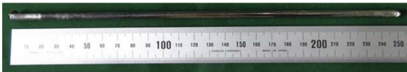
Figure 13.8. U-10wt%Zr-5wt%Mn fuel slug, fabricated by improved casting method
