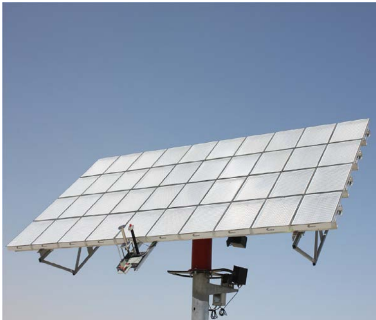
Figure 1.1.35. Photo of a test system consisting of 40 High Concentrating PhotoVoltaic (HCPV) modules with about 34% efficiency. This test system is a joint effort of Semprius (Durham, North Carolina, USA) and Siemens in collaboration with the Spanish Institute of Concentration Photovoltaic Systems (ISFOC) and the University of Madrid. Leading modules' manufacturers of conventional PV technologies achieved the maximum module efficiency of about 20% with mono-crystalline PV modules and about 16% with polycrystalline technology. Siemens press photo; copyright Siemens AG, Munich/Berlin, Germany
