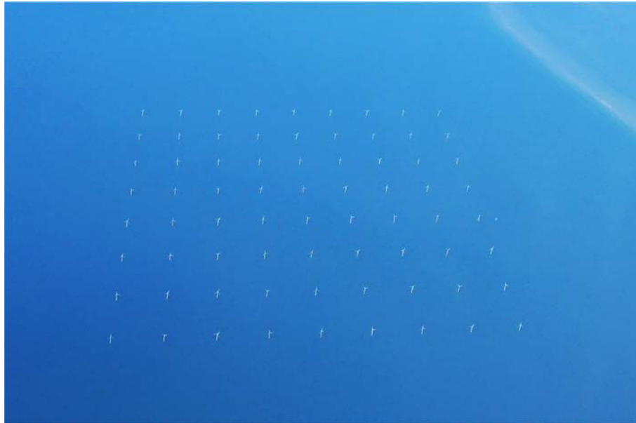
Figure 1.1.26a. Aerial view of 207-MW el off-shore Nysted (Rødsand) wind-turbine power plant (Denmark). The plant equipped with \sim 90 turbines 2.3-MW el each. The power plant provides enough power for more than 246,000 average Danish homes. Photo taken from Wikimedia Commons, author Plenz: https://en.wikipedia.org/wiki/Nysted_Wind_Farm#/media/File:Windpark_Nysted.jpg . Source: Wikipedia
