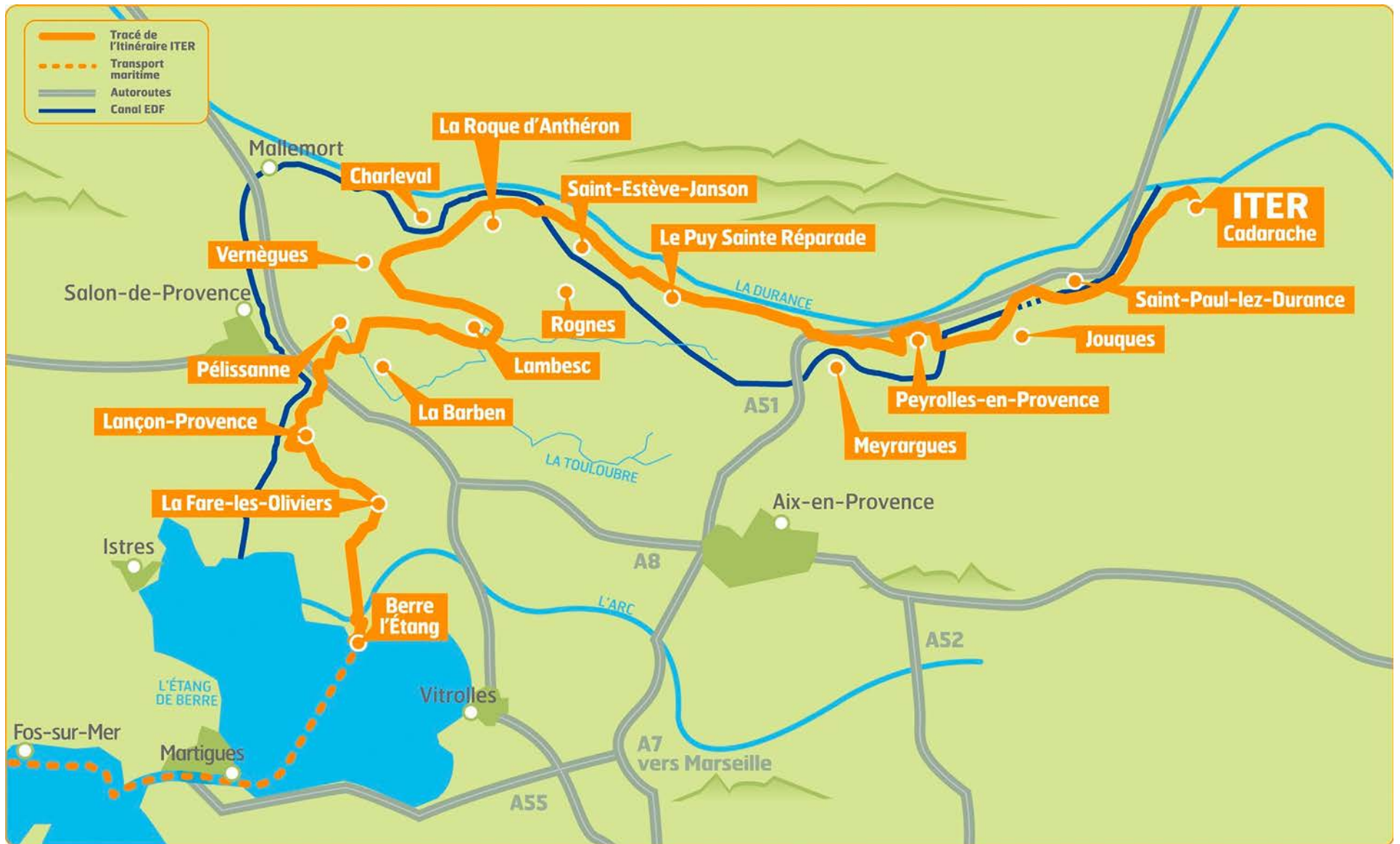
Figure 23.13. A map of the 104 km “ITER itinerary.” Some 10,000 ITER transports will use it, including 200 very exceptional convoys. The first of these HELs arrived on the ITER site on January 14, 2015. Credit: CEA-AIF
