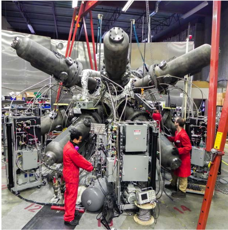
Figure 23.17. The machine built by General Fusion (Canada) is rather original; no vacuum vessel but a spherical tank filled with a liquid lead-lithium mixture; no superconducting magnets but an array of pistons to compress the plasma. Credit: General Fusion
