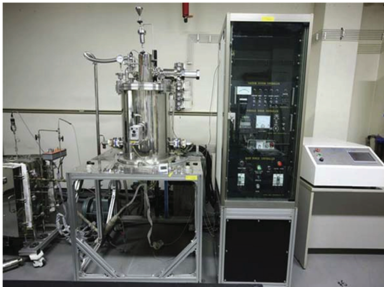
Figure 13.15. TRISO coating system
