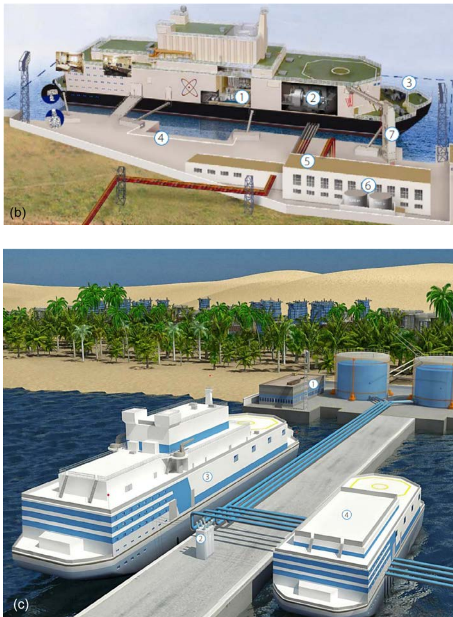
Figure 20.2.8, Cont'd (b) FNThPP layout with two KLT-40S reactors: 1—Reactors; 2—Steam-turbine power hall; 3—Underwater trench; 4—Waterside structures; 5—Heat point; 6—Hot-water tanks; 7—Switchgear and devices for electricity distribution and transmission to consumers. (c) Floating Nuclear Power & Desalination System (FNPDS) with KLT-40S Reactor(s) (artist image): 1—Coastal infrastructure; 2—Waterside structures; 3—Floating Power Unit (FPU); and 4—Floating Desalination Unit (FDU). (a) Courtesy of ROSATOM, photo by A. Bashkirov. (b) Courtesy of JSC “Afrikantov OKBM”: http://www.okbm.nnov.ru/upload/iblock/7c6/fc8drypg4s59sma16g1pajwe86j2tay1.pdf ; accessed Feb. 19, 2022. (c) Courtesy of JSC “Afrikantov OKBM”: http://www.okbm.nnov.ru/upload/iblock/7c6/fc8drypg4s59sma16g1pajwe86j2tay1.pdf ; accessed Feb. 19, 2022
