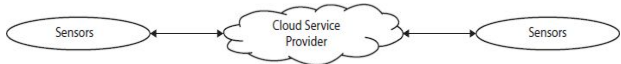
Figure 7.3 D-to-C communication model.
