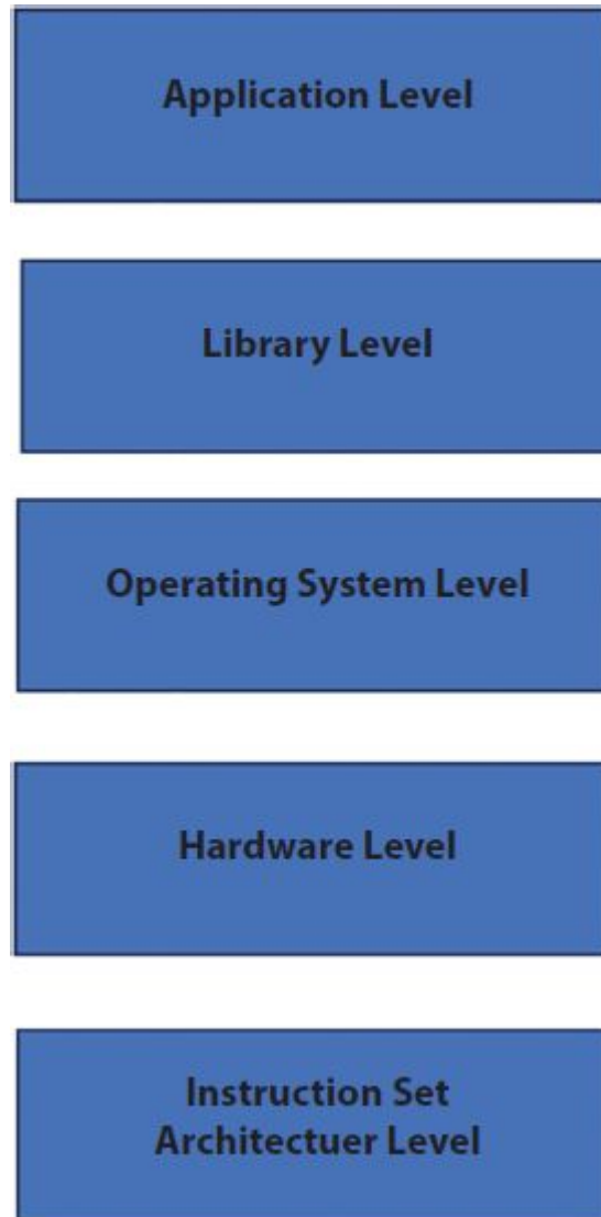
Figure 2.5 Different levels for implementation of virtualization [7].
