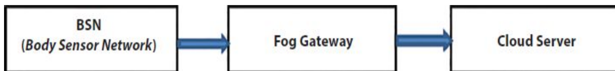
Figure 7.10 Fog computing architecture.
