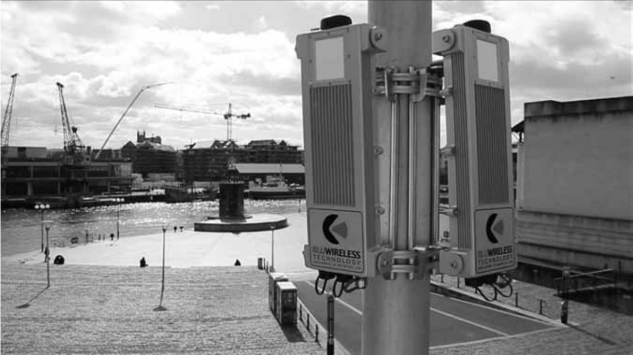
Figure 10.1 Outdoor lamppost-mounted 60-GHz Wi-Fi hot spot access point [9]. (Courtesy of Mark Barrett, Blu Wireless.)
