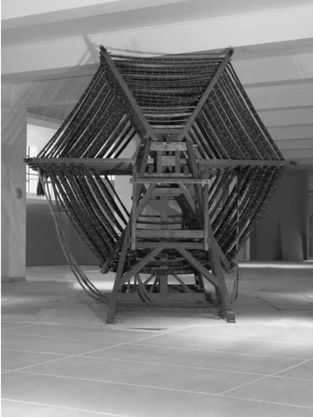
Figure 6.6 The Rugby tuning coil. (Courtesy of the Science Museum and Science Museum Picture Library.)
