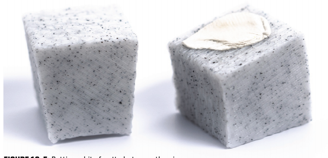
FIGURE 13-5: Putting a bit of putty between the pieces
