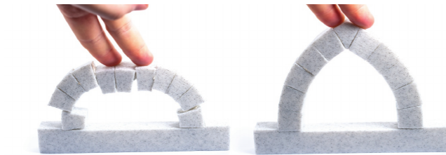
FIGURE 13-7: How arches collapse (or not)
