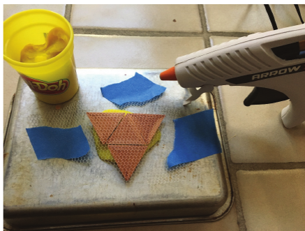
FIGURE 9-26: Setup for hot-gluing onto fabric.
