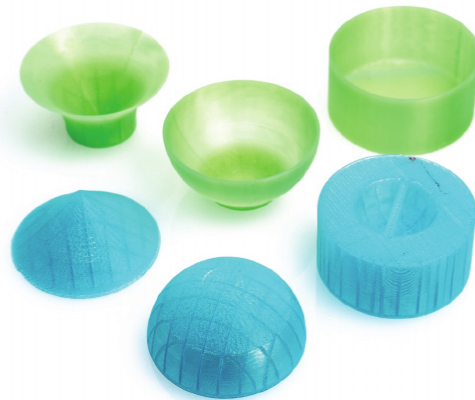
FIGURE 8-7: The cone, sphere, and cylinder molds (back row) and corresponding positive models (front row).
