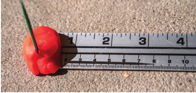
FIGURE 7-17: Using a ruler, toothpick, and clay as a gnomon
