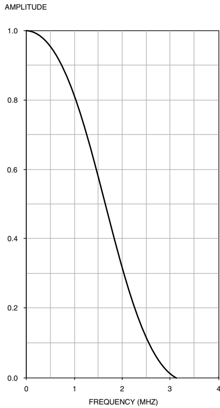
Figure 9.26. Typical 1.3-MHz Lowpass Digital Filter Characteristics.
