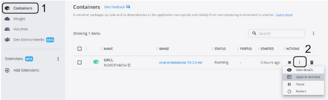
Figure A-15. To access a container’s shell, select the Container menu (1), click the three dots to access the “Show container actions” drop-down (2), and select the “Open in terminal” option
