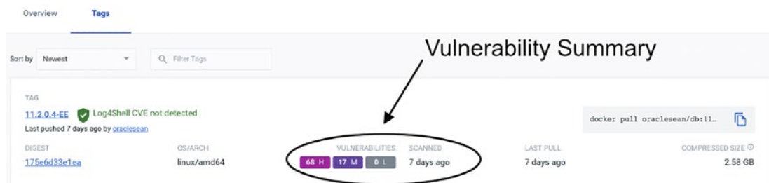
Figure 16-3. Image summary (from a private repository) for an Oracle 11.2.0.4 Enterprise Edition image. Scanning is an optional feature authors can request when uploading images to Docker Hub. Here, the image shows when it was last scanned and a summary of the high, medium, and low severity vulnerabilities present in the image
