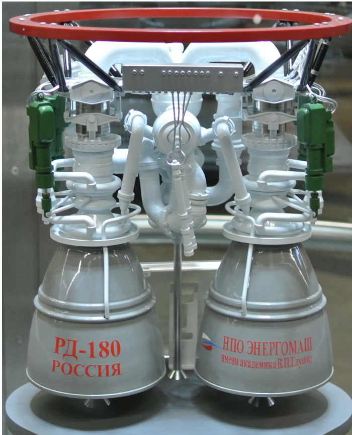
Figure 11.2 Energomash RD-180 rocket engine
