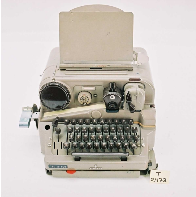
Figure 5.3 Teletype Type 68D from Siemens (Norsk Teknisk Museum)
