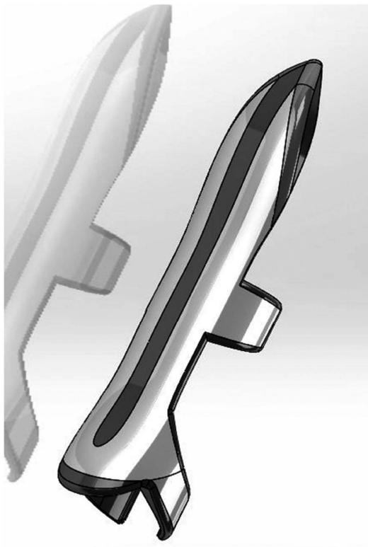
FIGURE 7.2 Customized design of finger splint.
