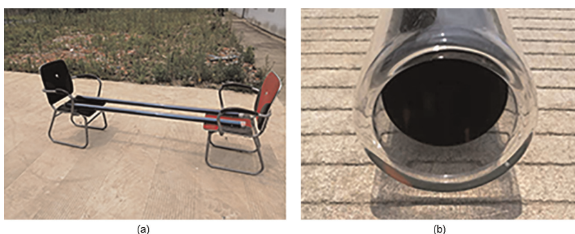
Figure 1. (a) Overview of the all-glass straight-through evacuated tube (b) Cross-section view of the inlet of the collector tube [51].
