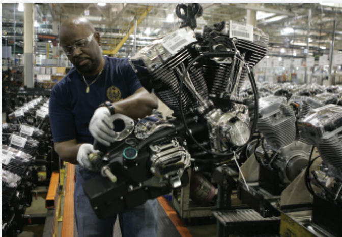
Engines are assembled in Memomonee Falls, Wisconsin, and placed in their own protective containers for shipment to the York facility. Upon arrival in York, engines are placed on an overhead conveyor for movement directly to the assembly line.
