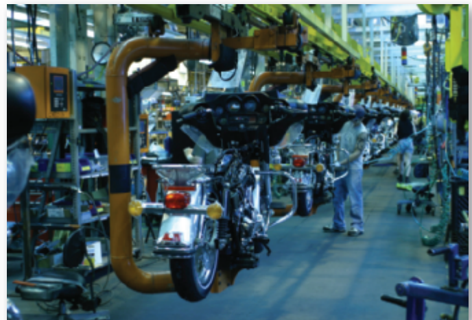
It all comes together on the line. Any employee who spots a problem has the authority to stop the line until the problem is corrected. The multicolored “andon” light above the line signals the severity of the problem.
