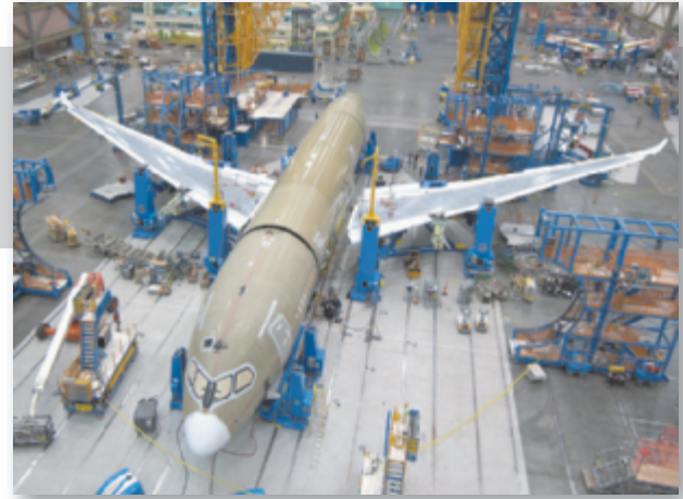
Components from Boeing's worldwide supply chain come together on assembly lines in Everett, Washington, and Charleston, South Carolina. Although components come from throughout the world, about 35% of the 787 structure comes from Japanese companies.
