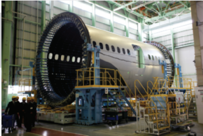
State-of-the-art composite sections of the 787 are built around the world and shipped to Boeing for final assembly.
