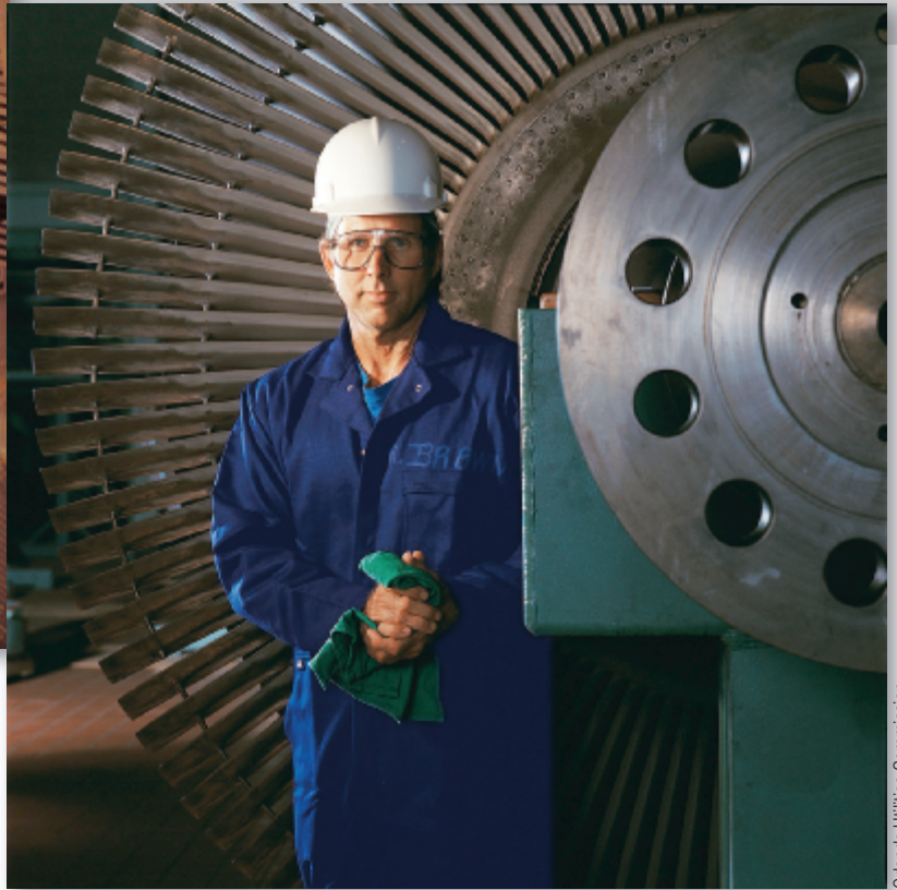
This inspector is examining a low-pressure section of turbine. The tips of these turbine blades will travel at supersonic speeds of 1,300 miles per hour when the plant is in operation. A crack in one of the blades can cause catastrophic failure.
