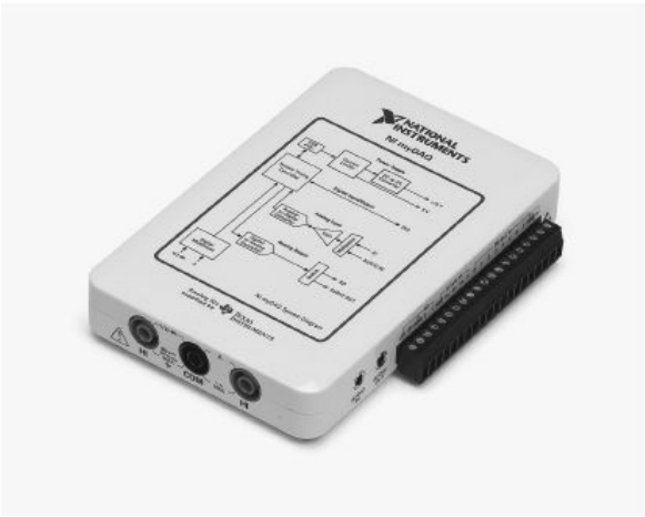
Fig. 2 The National Instruments myDAQ (left) and Digilent Analog Discovery (right) trainers use virtual instruments on a laptop to provide a low-cost base for most lab experiments.
