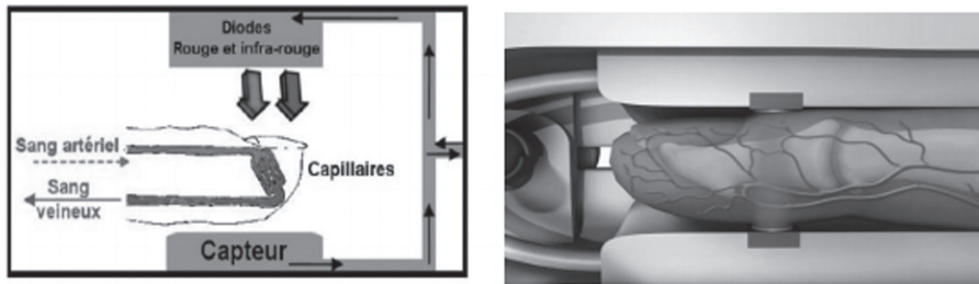
FIGURE 11.3 Principle of transmission/reception.
