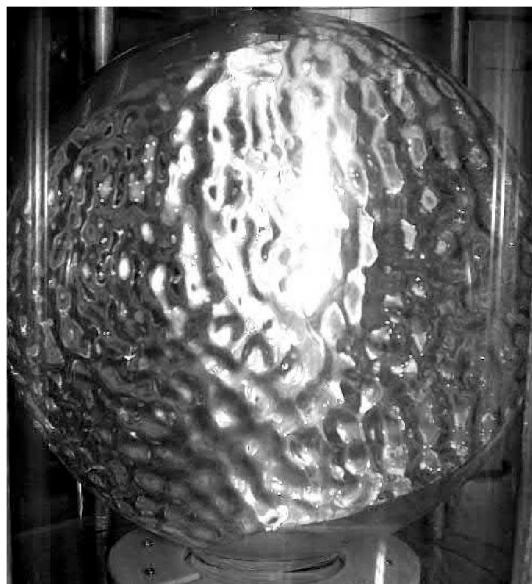
Figure 5.7 Capillary wave turbulence on the surface of a spherical container (of 15 cm diameter) filled with 20 cl of water. This result is obtained during a parabolic flight in free fall (Falcón et al., 2009). The fluid wets the inner surface of the sphere and forms a layer of spherical fluid. Purely capillary waves are then generated by vibrating the container. Credit: E. Falcon.
