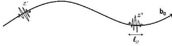
Figure 7.3 Propagation of two Alfvén wave packets along a quasi-uniform magnetic field that defines the parallel direction.
