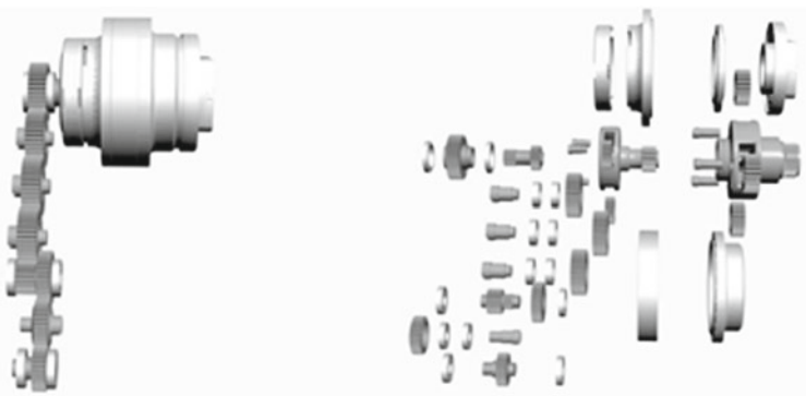
Fig. 4.16 Assembling and disassembling diagram of cutting part transmission gear
