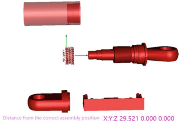
Fig. 4.20 Prompt diagram of correct assembly position
