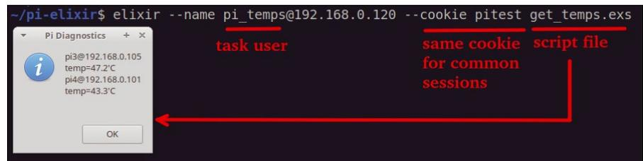
**Figure 6: Remote Pi CPU temperatures.**
