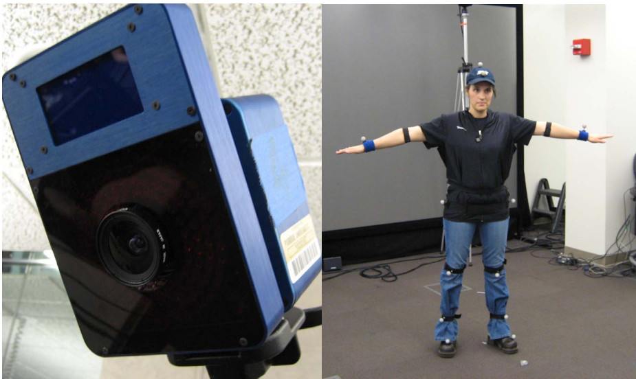
Fig. 1. One of six infrared cameras used in Envision Center's STT Motion Captor optical motion capture system (left) and a participant demonstrating a basic LED configuration (right)
