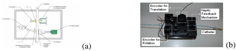
Fig. 3. (a): Mechanical structure of the MFB. The motion tracking module processes the translation and rotation motion of the catheter/guidewire. (b): Physical set of MFB.
