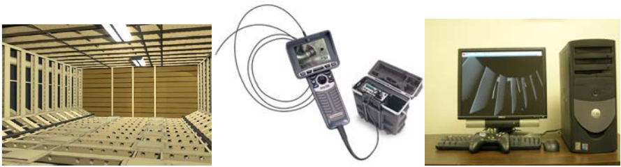
Fig. 3. Enhanced VR cargobay model ( left ), actual video borescope ( center ) and virtual borescope simulator ( right )
