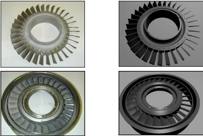
Fig. 4. Engine blades modeled (right) from the actual engine (left)
