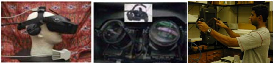
Fig. 1. Hardware used to develop and test the simulators including the HMD and 6DoF mouse (left), the HMD eyetracking system (center) and the touch screen WindowVR unit (right)
