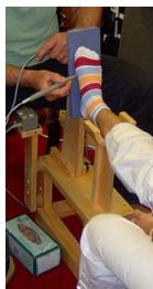
Fig. 1. The leg support was built of wood with no metal parts (e.g., nails or screws), so as to not interfere with the transmitter's electromagnetic field
