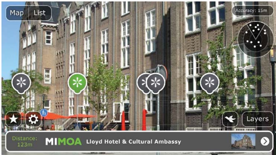
Figure 5.24 Screenshot of Layar’s application for Android that allows users to combine a video camera view of the world with useful information shown as a digital layer on top of the screen view
