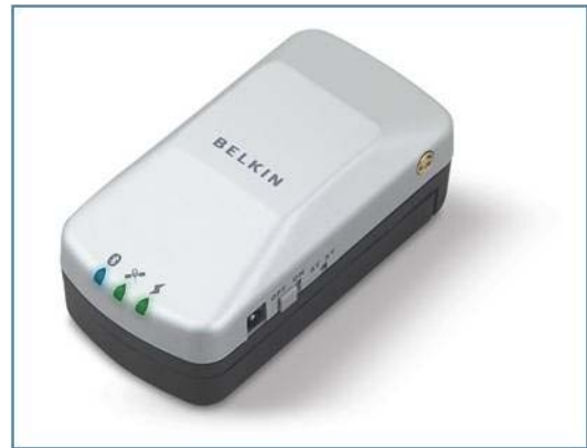
Figure 2.4 A Belkin Bluetooth GPS device that can be connected to a mobile phone to provide additional GPS functionality
