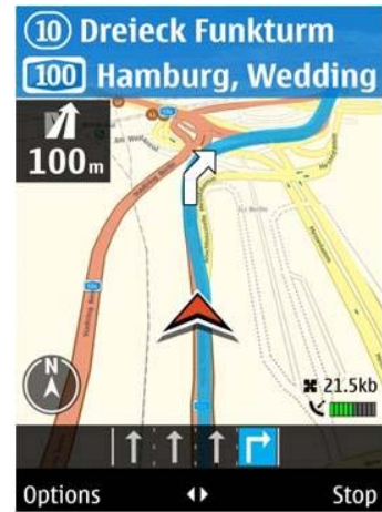
Figure 5.3 An example screenshot of Ovi Maps' Drive in-car routing on a mobile phone screen providing real time, turn-by-turn navigation using GPS
